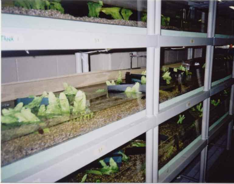
Figure 3.2 Arrangement of 548.6cm x 50.8cm x 15cm population tanks.
