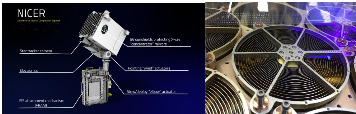
Figure 1.3: Diagram of the NICER instrument attached to the ISS on the left and close up of one of the detectors on the right. 40
