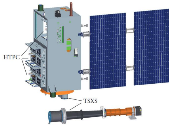
Figure 1.4: Diagram of the XPNV-1 Satellite. A mock-up of the TSXS detector is provided. [73]
