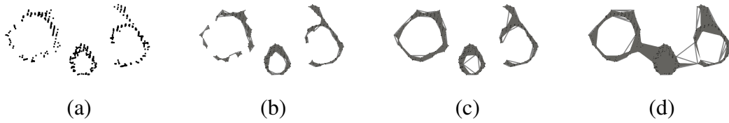
Figure 3.18: Examples of built \alpha -complexes of stem points from three close trees in Figure 3.17. (a) Stem points with p.h < 1m . Built 2D \alpha -complexes of stem points with (b) \alpha = 0.05m , (c) \alpha = 0.1m , and (d) \alpha = 0.15m .
