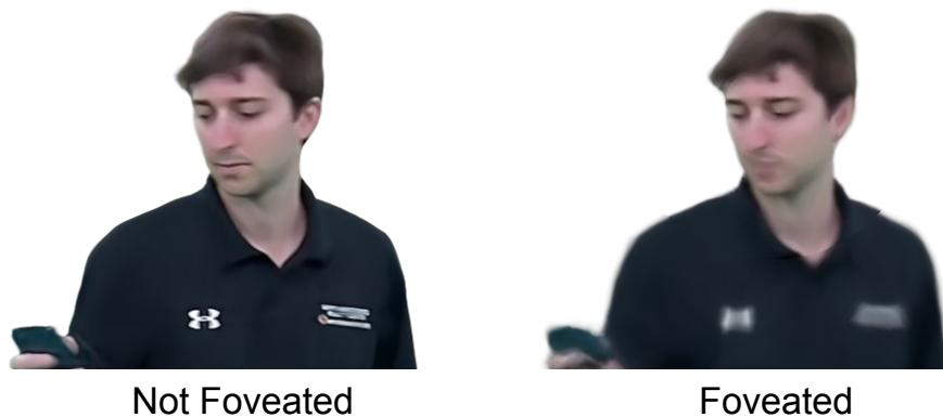
Figure 3.7: An example of foveated rendering from our progressive multi-scale LFN. Foveated rendering generates peripheral pixels at lower levels of detail to further improve performance in eye-tracked environments. In this example, foveation is centered over the left eye of the subject.
