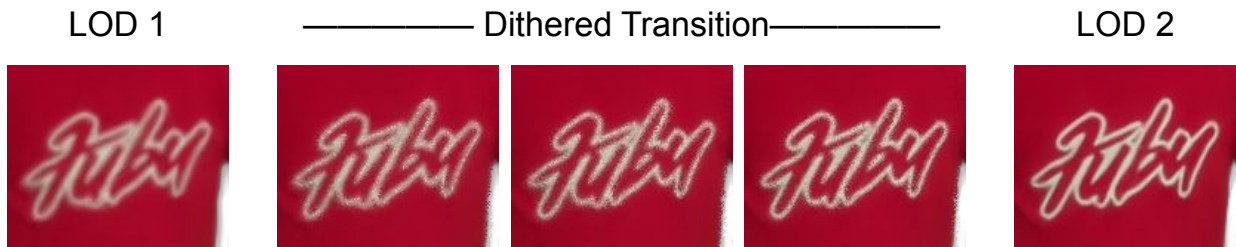
Figure 3.6: With per-pixel level of detail, dithering can be applied to transition between levels of detail.
