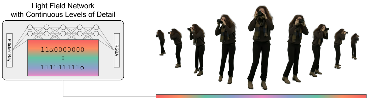
Figure 4.1: Our light field network features continuous levels of detail, enabled by training with summed-area table filtering and saliency-based importance sampling. Continuous levels of detail enable the interactive streaming of light fields with smooth transitions and finely tuned adaptivity.
