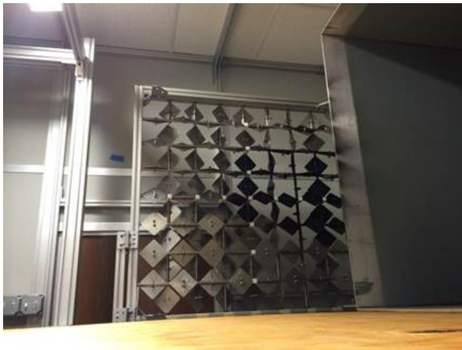
Figure B.1: ATG turbulence grid
