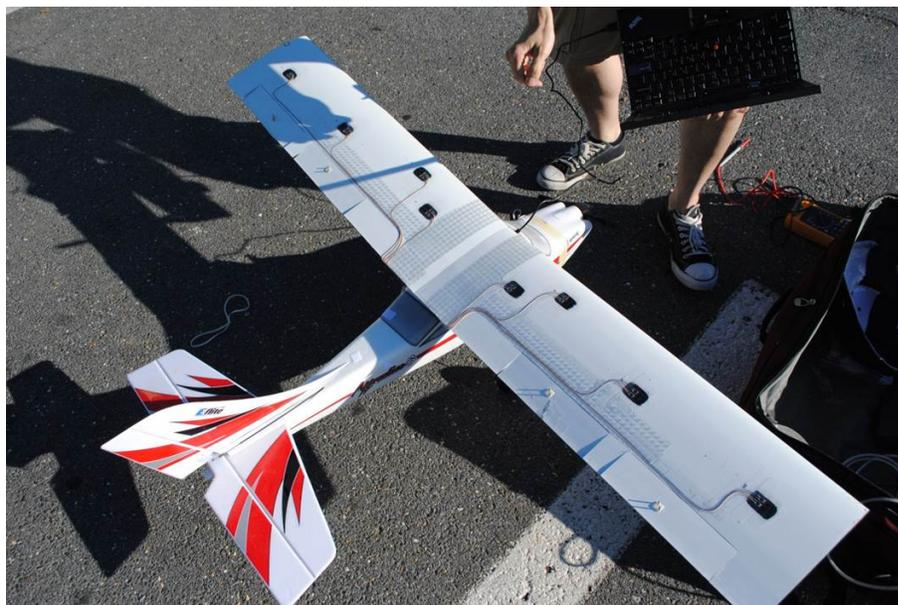
Figure 4.66: Apprentice aircraft and ground station during flight test preparation
