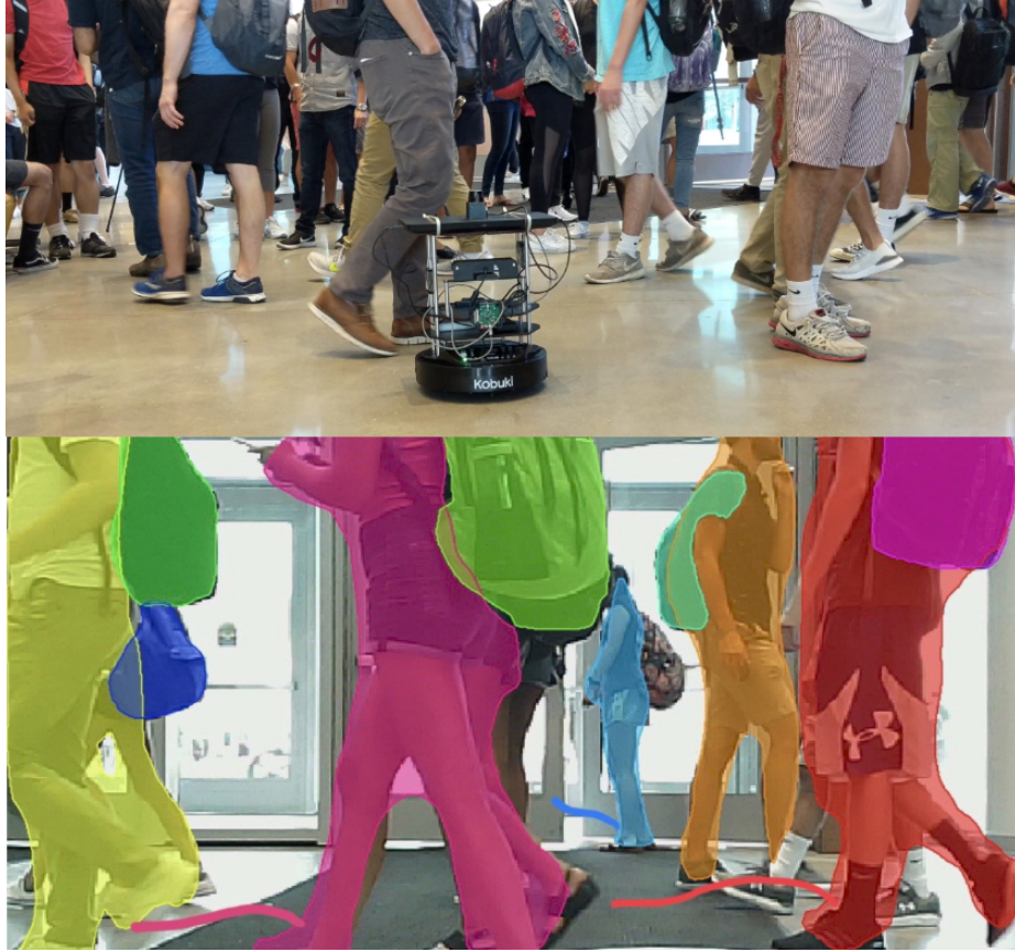
Figure 2.1: [Top] DenseCAvoid implemented on a Turtlebot navigating through a dense crowd. [Bottom] We explicitly track and predict pedestrian motions (marked for three pedestrians) and use it to train a Deep Reinforcement Learning-based collision avoidance policy. Our network implicitly learns to reduce the occurrence of the freezing robot problem and generates smooth robot trajectories in dense crowds.
