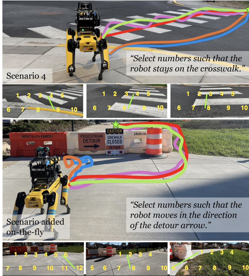
Figure 5.2: [Top] : The trajectories of a Spot robot crossing the road when using CoNVOI with GPT-4v [237] (in green), CoNVOI with Gemini [240] (in purple), teleoperated by a human (in red), GA-Nav [18], and DWA [29]. CoNVOI navigates the robot on the crosswalk by understanding the environmental context. [Bottom] : The trajectories when the Spot robot navigates to a goal beyond a blockade. While using CoNVOI, handling such scenarios can be added on the fly using a simple text prompt without any reformulation. The RGB images from the robot are shown with CoNVOI’s multi-modal visual marking (numbers in yellow). GPT-4v/Gemini is queried with the marked image and a context-based text prompt in quotes, and it returns the green reference path that follows explicit, and implicit social rules, and human-like preferences during indoor and outdoor navigation.
