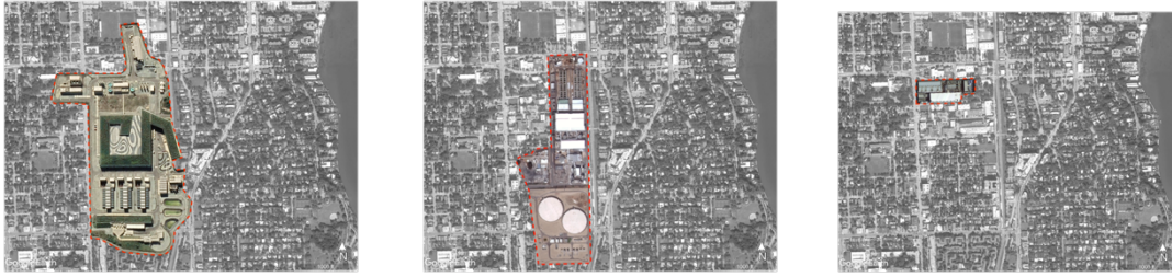
Fig. 10: Profiled desalinization plants superimposed on site. (Left) Victoria, Australia desalination facility (78 acres ; (Middle) Sorek, Israel desalination plant (55 acres), (Right) Carlsbad, California desalination plant (9 acres). Images by author.
