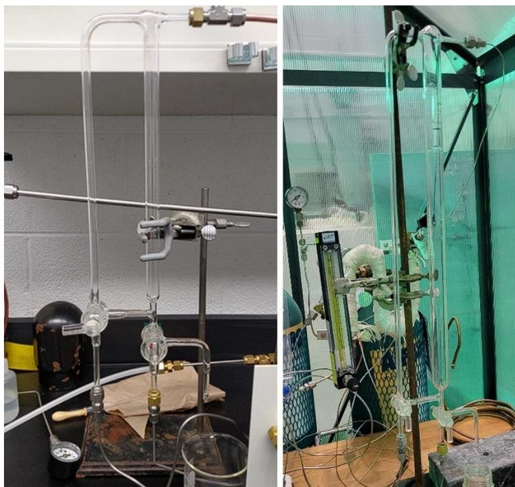
Figure 46. Pictures of the original 20mL glass sparging apparatus (left) (adopted from (Dietz, et al., 2021)), and the larger 150mL glass sparging apparatus custom made for this project (right).
