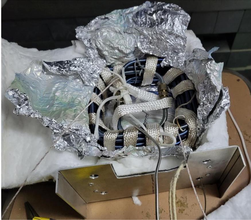
*Figure 43. Photograph of the zirconium alloy irradiation cell tubing, wrapped in heating tape, along with a layer of aluminum foil and of fused silica batting insulation.*
