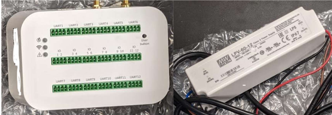
Figure 2.3. Data logger (left) and power supply (right) used.
