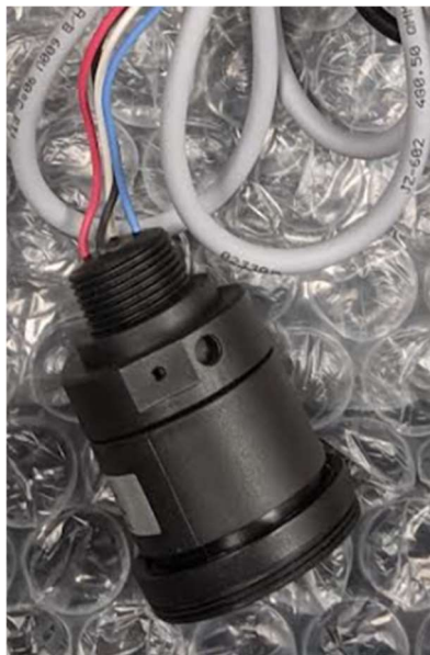
Figure 2.1. Image of the housed NDIR sensor provided by Company X.
