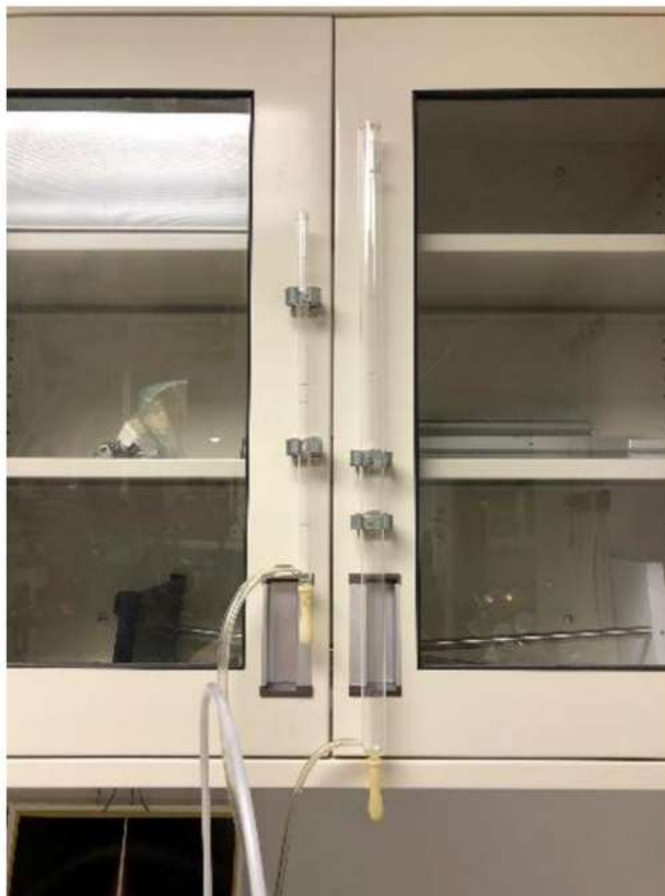
Figure 2.7 Image of soap bubble flow meter used for calibration.
