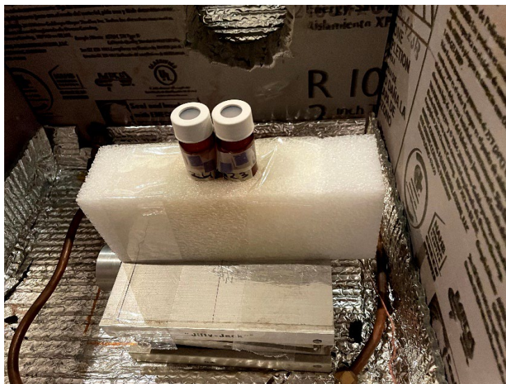
Figure 22. The inside of the “hot box” insulated irradiation chamber used for high temperature irradiations.
