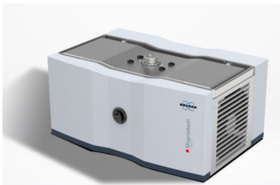
Figure 26. Bruker Alanine Dosimeter Reader. Alanine strips were inserted into the middle cavity after irradiation.
