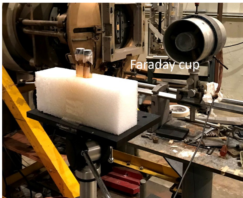
Figure 27. Faraday cup in reference to the sample placement.
