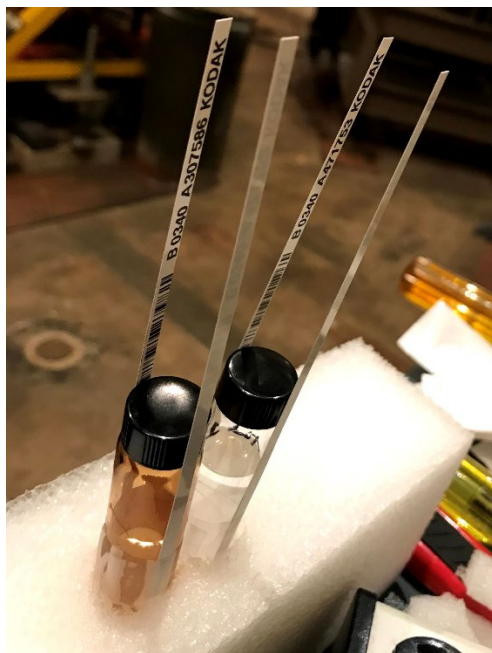
Figure 25. Alanine strips placement for dosimetry measurements.
