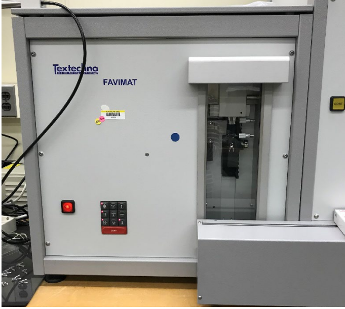
Figure 32. FAVIMAT single-fiber tester used for the mechanical testing of aramid fibers. Inset on the right shows the set-up, with a mini spring clamp placed on the end of the fiber which kept them taut.
