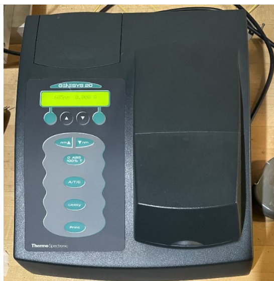
Figure 29. Visible Spectrophotometer used for radiochromic film dosimetry.
