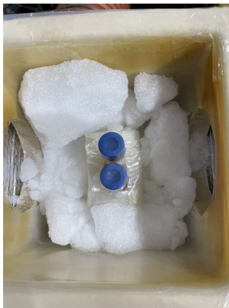
Figure 23. The inside of the cooler used as an insulated irradiation chamber for conducting the irradiation experiments at sub-ambient temperature.
