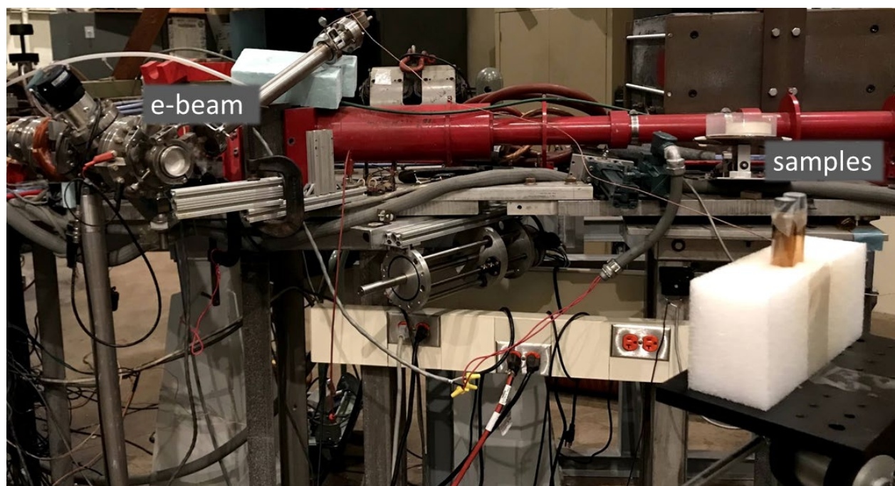
Figure 21. Set-up of sample irradiation in front of the e-beam.
