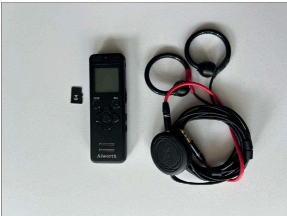
Figure 2: Recording materials used for initial dataset construction. Handheld flash-based recorder (Left) and SonicPresence SP15 Binaural Over-Ear Microphone
