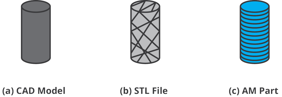
Figure 4.6: Process for Manufacturing AM Parts
