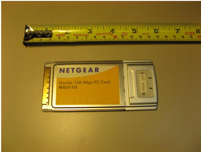
Figure 5.3: Netgear Atheros-based network card
