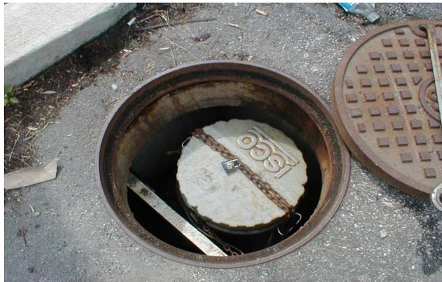
Figure 3.7. Isco, Model 6712 Portable Sampler installed in storm drain on west side of Route 1 at Mt. Rainier, MD monitoring site
