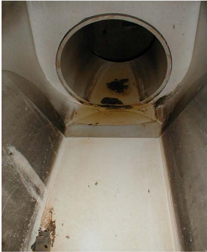
Figure 3.6. Palmer-Bowlus 24" flume installed in storm drain on west side of Route 1, Mt. Rainier, MD monitoring site
