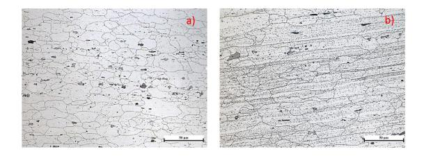
**Figure 9.** Al<sub>3</sub>Mg<sub>2</sub>  $\beta$  phase increases as the aging temperature increases and under a constant aging time. (a) Sample U3 aged at 100°C for 168 hours. (b) Sample U7 aged at 150°C for 168 hours
