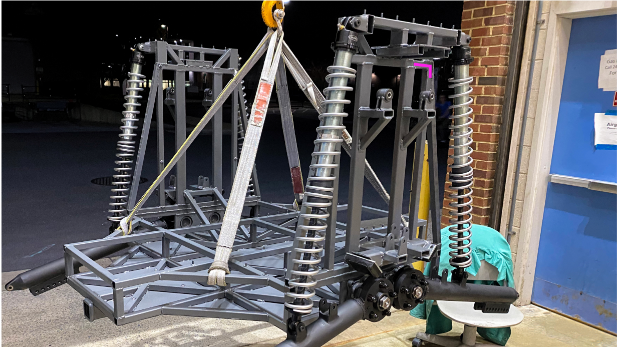
Figure 2.26: Chassis after modification to remove old mounts and create new structure
