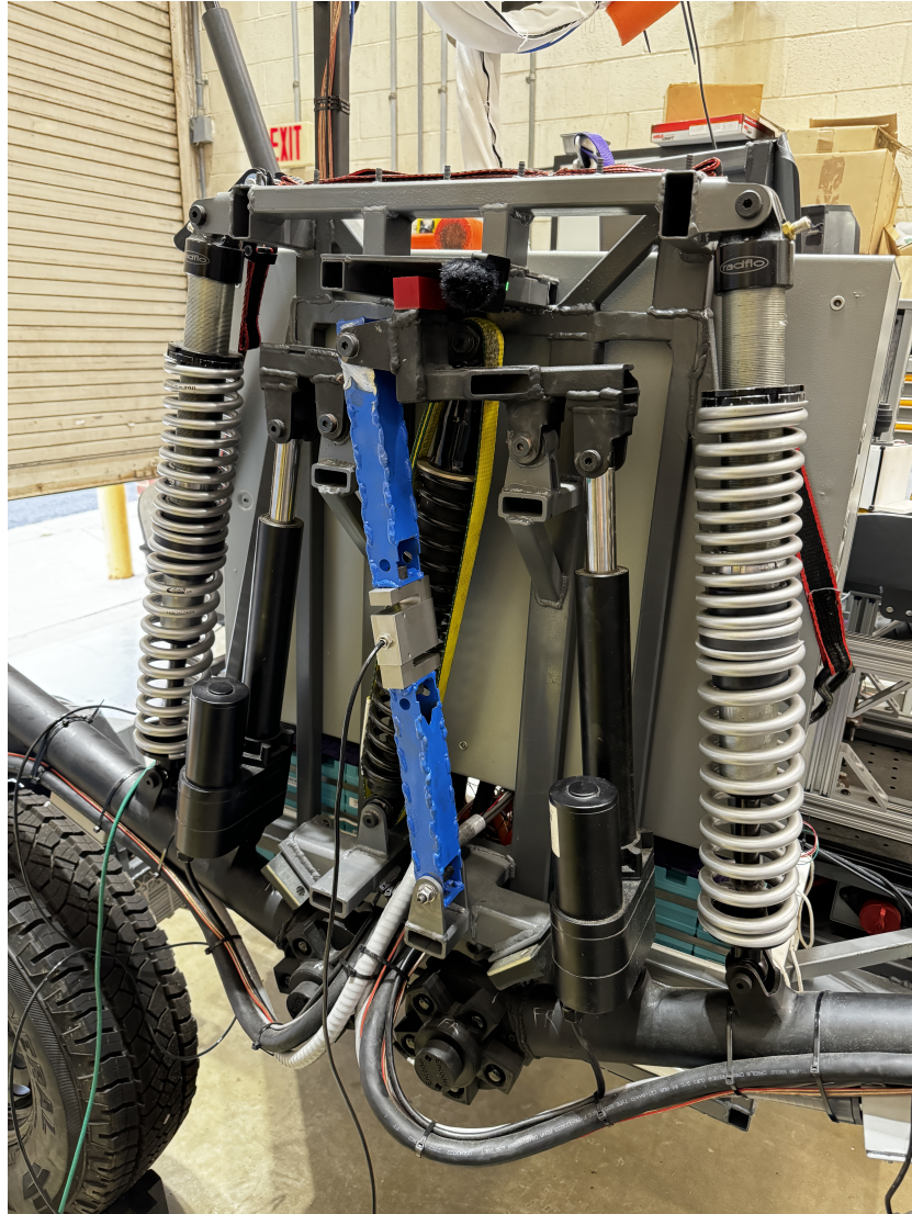
Figure 4.1: Load cell integration into the front-right suspension system on VERTEX, replacing the series elastic element.
