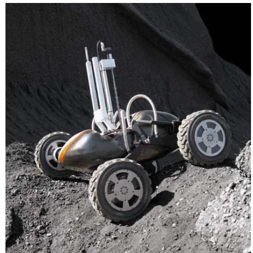
Figure 1.11: CMU’s SCARAB rover conforming to terrain during field trials [25]
