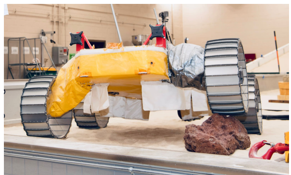
Figure 1.7: NASA's VIPER rover demonstrating suspension articulation, leveling chassis on a rock in a testbed [18]
