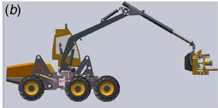
Figure 1.14: AWLFC concept showing a separated, active articulated rocker-bogie style logging suspension concept [30]
