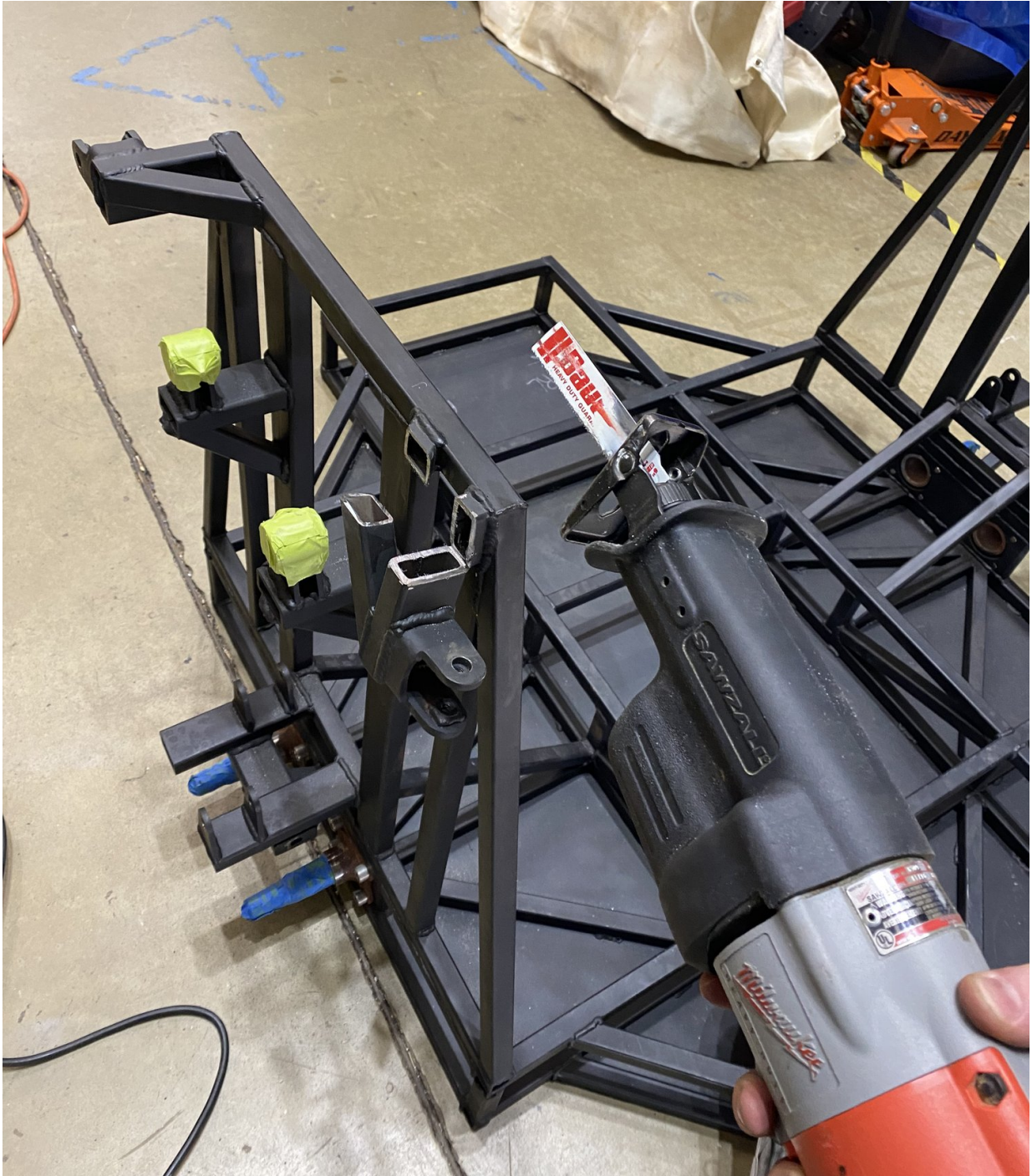
Figure 2.25: Heavy chassis modifications required for upgraded suspension including removal of old structure and welding of new supports to support dual-rate spring dampers.
