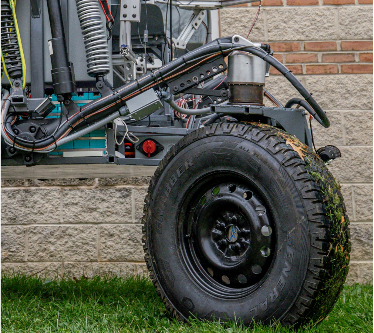
Figure 2.18: VERTEX rover during its first field excursion, showing the caster angle adjustment system is in its minimum angle state.
