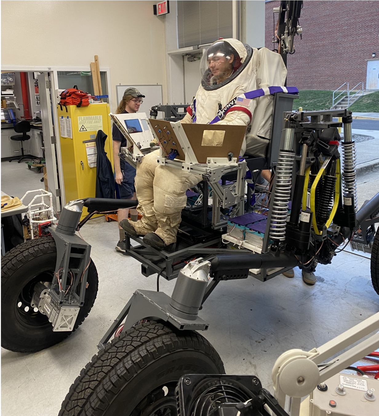
Figure 2.24: Dual rate spring modification exhibiting lack of rebound and controllability at steady state conditions due to higher than expected sprung mass during electronics integration phase. Top rate 150 lb/in, bottom rate 200 lb/in. Increasing the dual-rate damper's preload returned the system to positive static stability.
