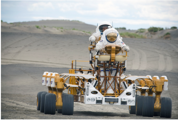
Figure 1.25: NASA's Chariot, a full-size analogue vehicle, in testing with two test subjects [21]
