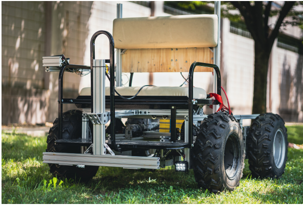
Figure 1.1: SSL's Raven rover, built as an astronaut transport rover for analogue field testing.
