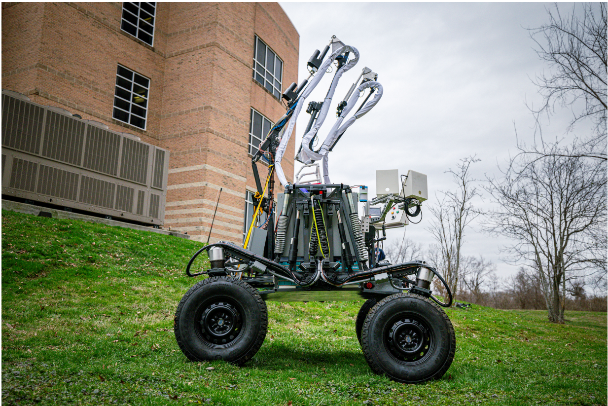
Figure 2.2: VERTEX roving vehicle side profile showcasing suspension system. The fully independent suspension features a series-elastic actuator with a parallel dual-rate spring damper.
