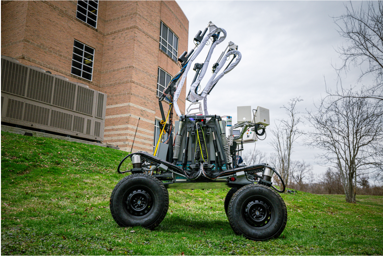
Figure 1.17: Side profile of the VERTEX rover carrying the umbilical-tending arm (ARMLiSS), featuring its high range of motion articulated suspension system with passive spring damping and a fine-detail Lagrangian dynamics scheme. The next sections examine the analytical and computational tools that have been deployed historically, clarifying why new techniques and approaches are necessary for vehicles like VERTEX.
