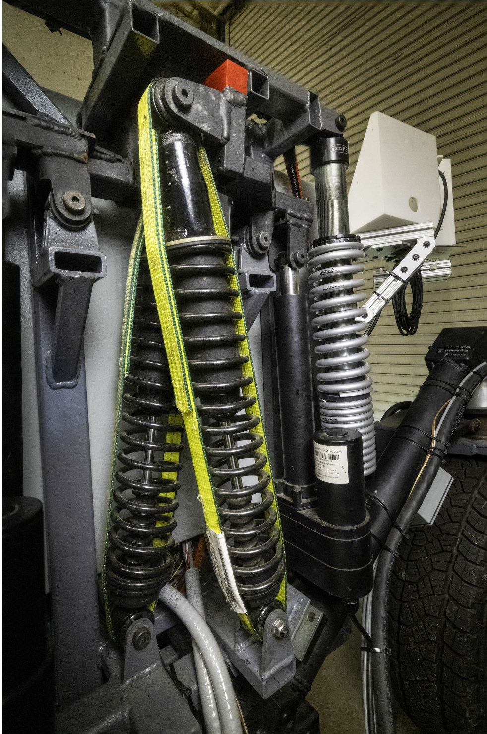
Figure 3.11: Bushing elements shown in a perspective image of the suspension system. The bushings are seen at the top and bottom connectors for the series elastic element and at the central pivot point between the linear actuator and the SEE.
