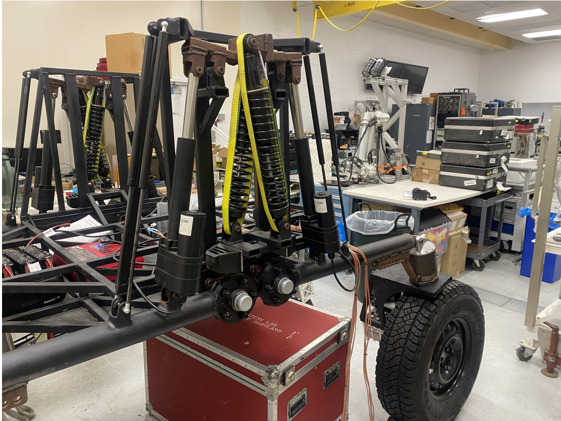
Figure 2.4: Initial suspension system during preliminary VERTEX build stages with the first suspension system.
