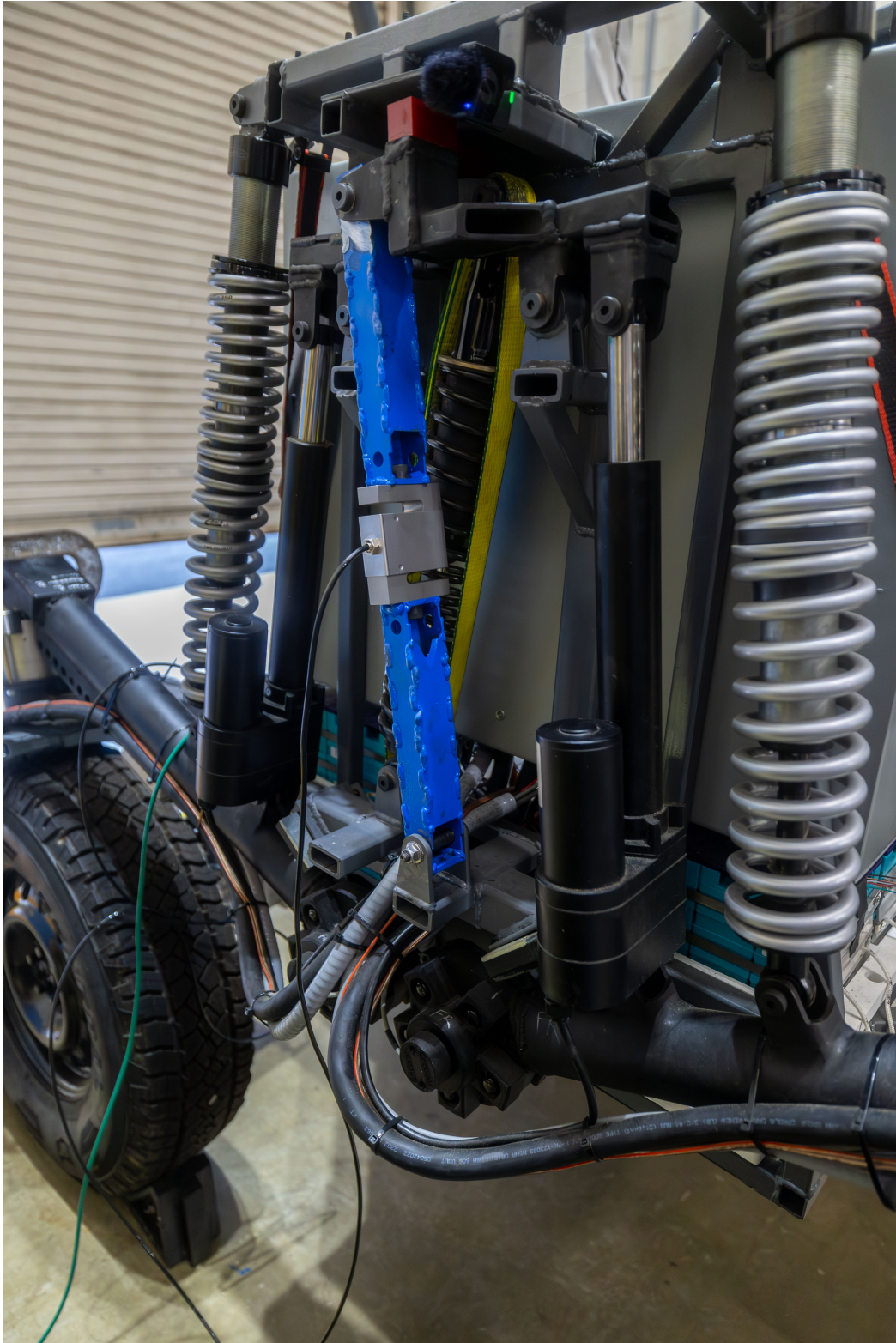
Figure 2.27: Compression/tension load cell sensor replacing the series-elastic element in the VERTEX suspension system
