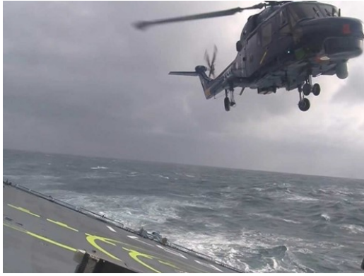
(a) Hover over a sloped ship deck [30].
