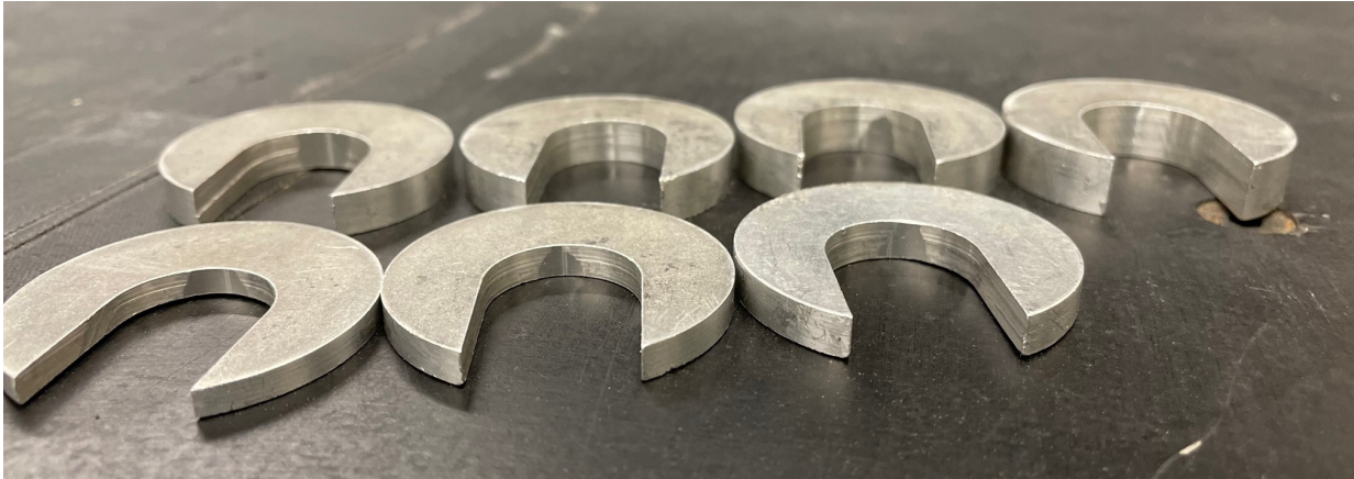
Figure 2.3: Measurement spacers used when adjusting blade pitch.
