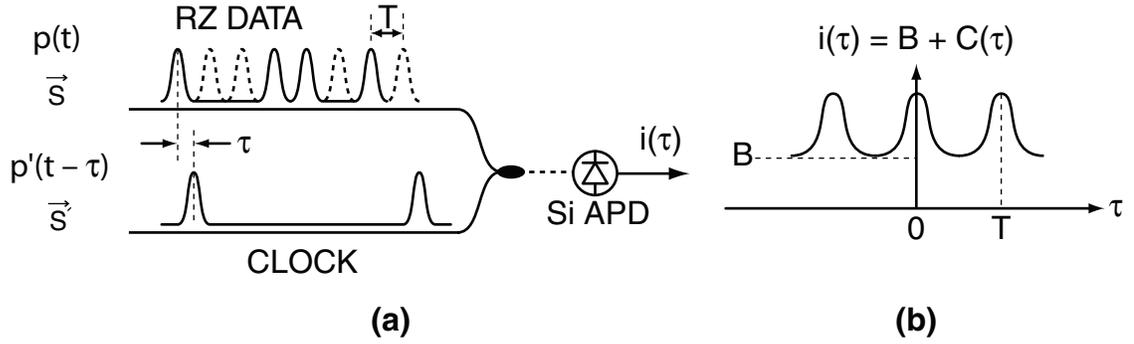
**Fig. 2.16:** Schematic of cross-correlation measurement produced by two-photon absorption. (a) Two optical signals are combined and directed to the silicon detector. (b) The time-averaged photocurrent  $\langle i(\tau) \rangle$  is comprised of a cross-correlation signal  $C(\tau)$  on top of a constant background level  $B$ .
