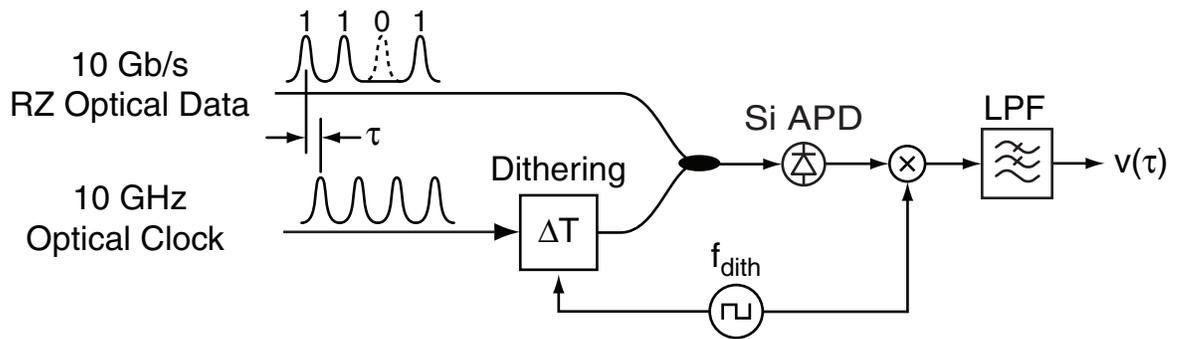
**Fig. 2.28:** Diagram of dithering clock recovery experiment.
