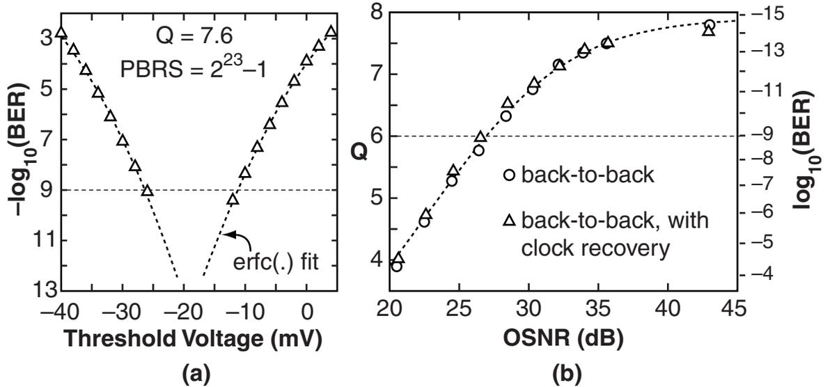
**Fig. 2.11:** (a) Measured bit-error-rate vs. decision threshold for the case when  $Q = 7.6$ . (b) Measured back-to-back  $Q$  vs. OSNR for the system depicted in Fig. 2.10, with and without clock recovery, showing no appreciable penalty.
