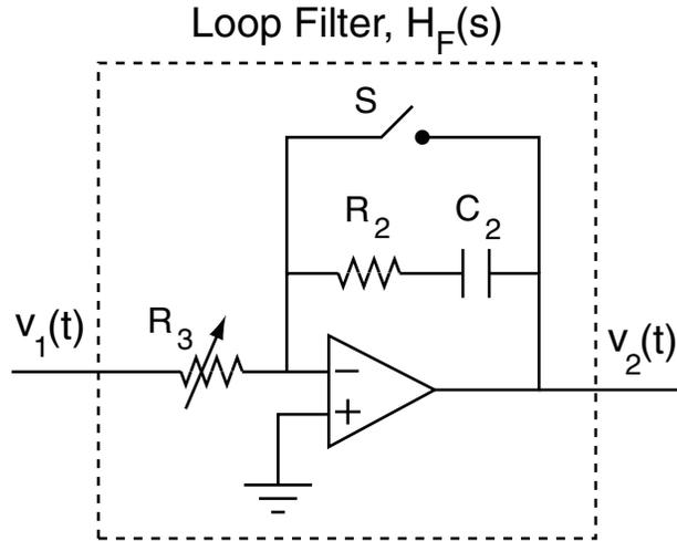
**Fig. A.4:** Loop filter circuit.
