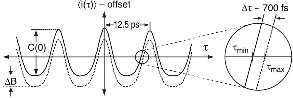
**Fig. 2.17:** Measured minimum and maximum cross-correlation signals obtained by adjusting the data polarization, when the clock is circularly polarized. Changes in the polarization state produce a change  $\Delta B$  in the background level, which can shift the zero-crossing point by as much as 700 fs.
