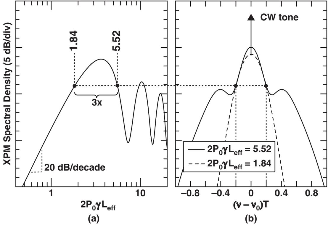
**Fig. 3.9:** (a) Calculated XPM spectral power at an offset frequency of  $(\nu - \nu_0) = \pm 0.2/T$ , as a function of  $2P_0\gamma L_{\text{eff}}$ . The two labeled points show that  $\gamma$  can change by  $3\times$  without changing the XPM spectral power. (b) Calculated XPM spectra for the two points labeled in (a), showing the crossing points at  $(\nu - \nu_0) = \pm 0.2/T$ .
