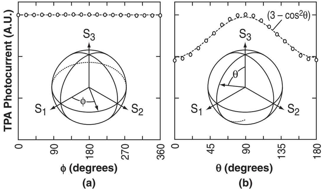
**Fig. 2.12:** Measured photocurrent produced by two-photon absorption as a function of the polarization state. (a) The photocurrent produced by two-photon absorption is the same for all linear polarization states. (b) When the polarization state changes from linear to circular, the photocurrent decreases by a factor of approximately  $2/3$ .
