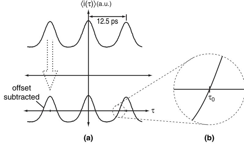
**Fig. 2.7:** (a) Measured cross-correlation between 10 GHz clock and 80 Gb/s data before and after the offset is subtracted. (b) Magnified view of cross-correlation, showing the zero-crossing location.
