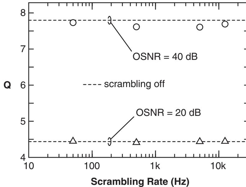
**Fig. 2.22:**  $Q$  as a function of the speed of polarization scrambling, measured at two representative OSNR levels. The dashed line indicates the value of  $Q$  obtained without scrambling.
