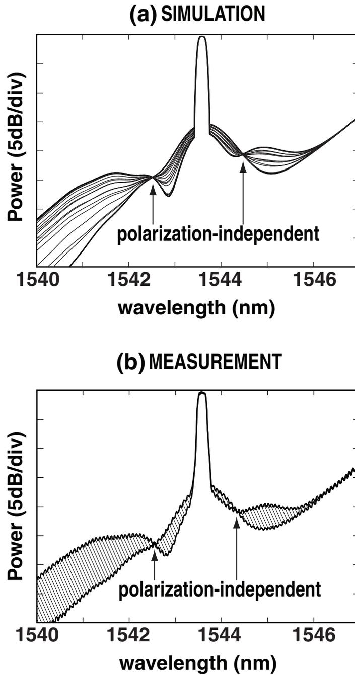
**Fig. 3.8:** (a) Simulation results and (b) measurements at 150 mW pump average power. Good agreement between the two can be seen. Polarization-independent points on both sides of the CW probe can be predicted with our numerical simulation.
