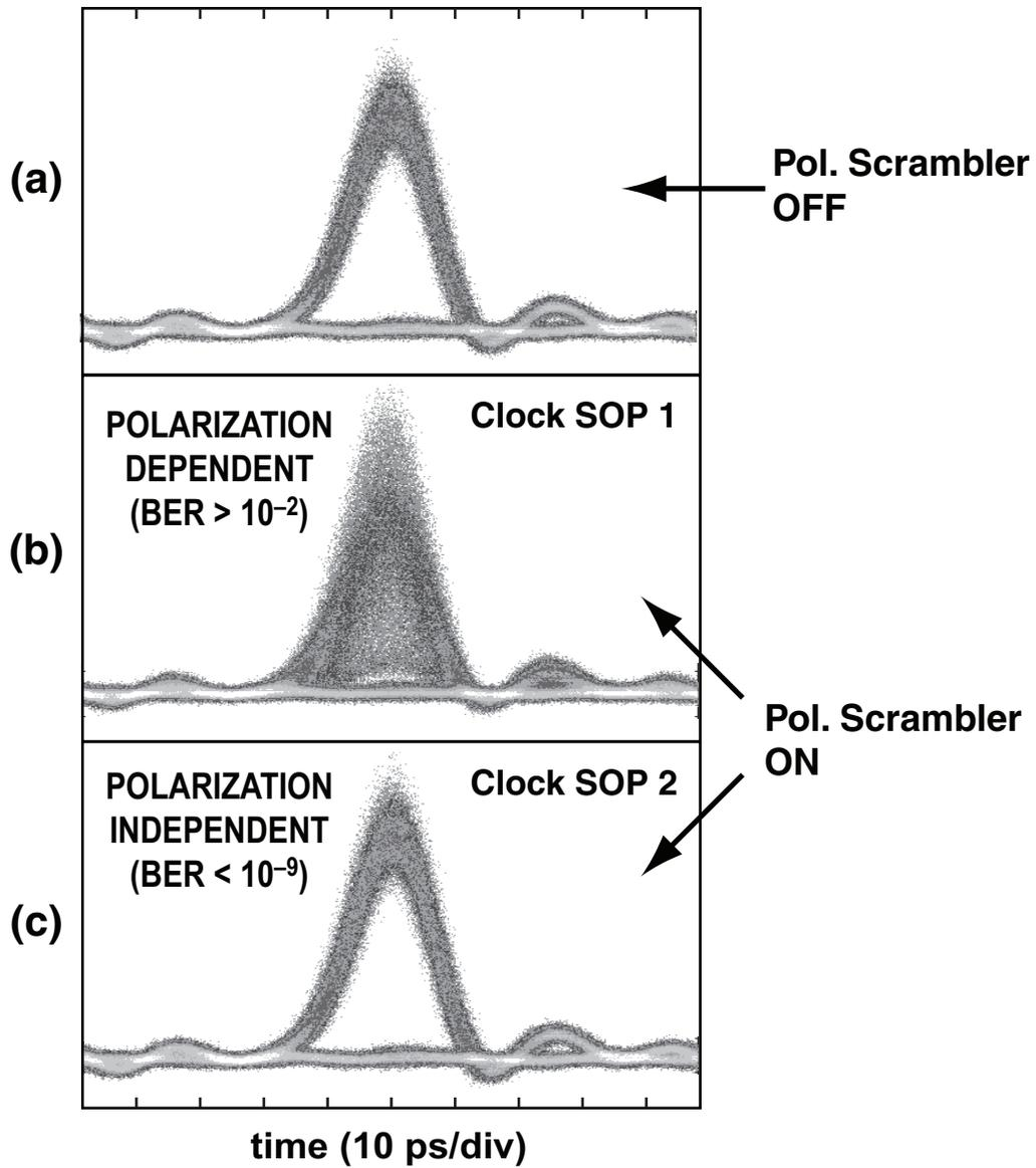
**Fig. 3.25:** (a) 10 Gb/s demultiplexed data eye diagram when the polarization scrambler is off. (b) data eye diagram when polarization scrambler is on and clock polarization is adjusted to the worst state. (c) data eye diagram when polarization scrambler in on and clock polarization is adjusted to the best state.
