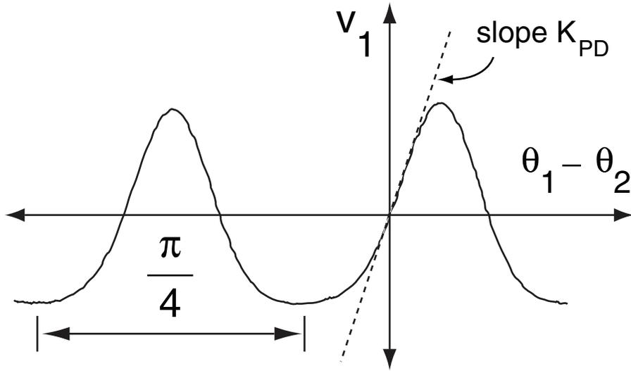
**Fig. A.3:** Measured error signal of the PLL as a function of the phase difference between the two optical inputs. Phase-detector sensitivity  $K_{PD}$  can be calculated by finding the slope of the tangent to the curve at the origin.
