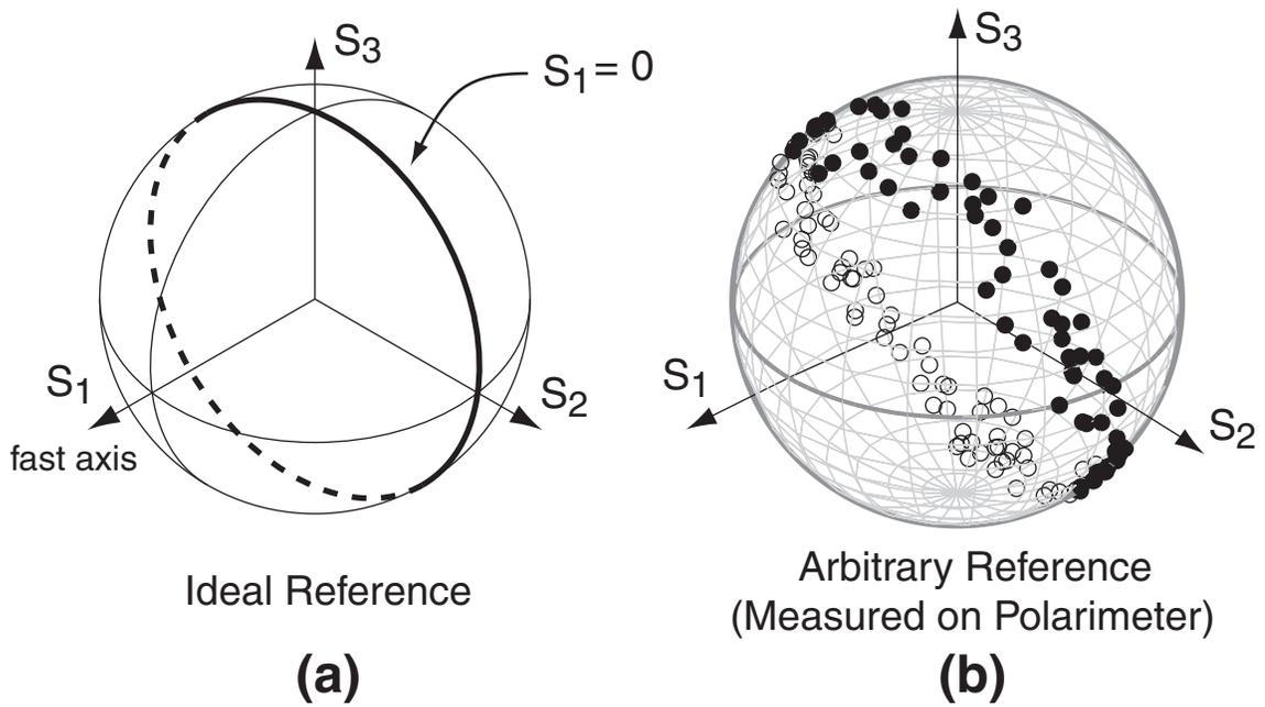
**Fig. 3.27:** (a) The circle including all pump polarization states that lead to polarization-independent XPM shown on Poincaré sphere with ideal reference axes. (b) The S parameters for the clock polarization states that lead to bit-error-rates  $< 10^{-9}$  while data polarization is scrambled (reference for the Poincaré sphere is arbitrary due to measurement issues.)
