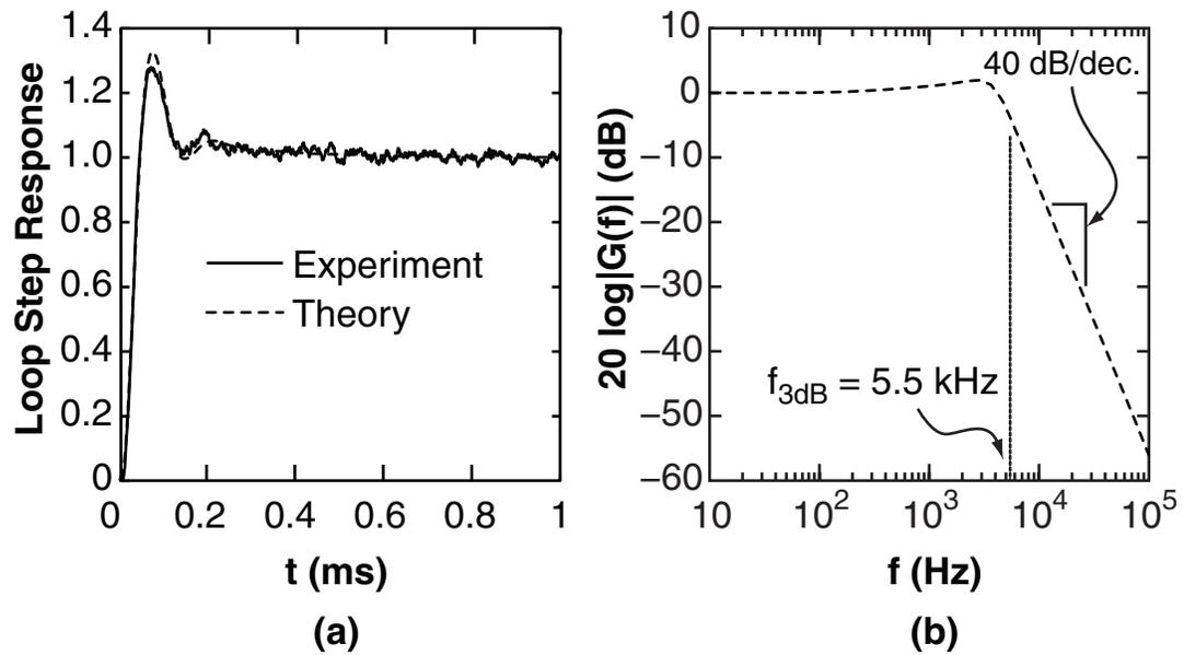
**Fig. 2.8:** (a) Measured and theoretically-predicted step-response of the phase-locked loop clock recovery system. The system exhibits a rise time below 0.20 ms. (b) The corresponding closed-loop spectral response of the phase-locked loop, showing a bandwidth of 5.5 kHz.
