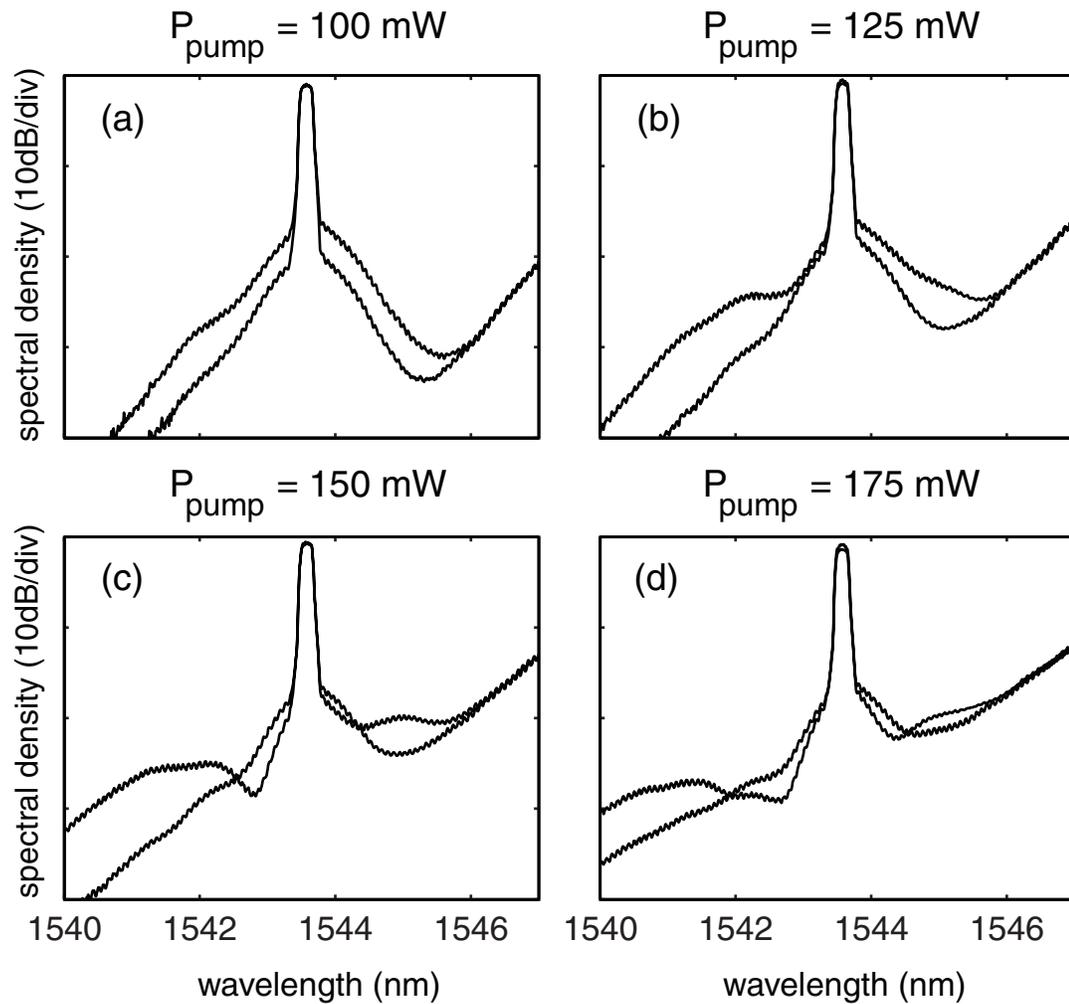
**Fig. 3.7:** Polarization dependence of XPM spectral density for CW probe signal and pulses pump signal. Parts (a)-(d) plot two extreme cases of probe polarization states for four difference pump average power levels. (RBW = 0.2 nm)
