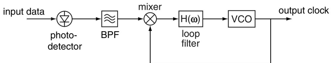
**Fig. 2.1:** Diagram of electrical clock recovery system.
