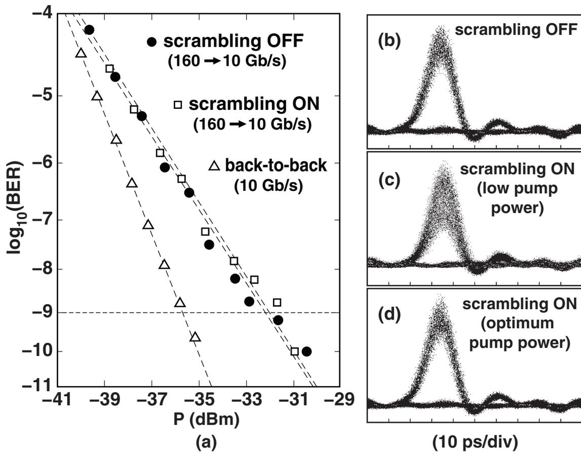
**Fig. 3.17:** (a) Bit error rate vs. received power for the 160 Gb/s demultiplexer, showing little penalty when polarization scrambling is enabled. Measured eye diagram of demultiplexed 10 Gb/s data while (b) polarization scrambling is disabled, (c) polarization scrambling is enabled but pump power is lower than optimum level and (d) polarization scrambling is enabled and optimum pump power is used.
