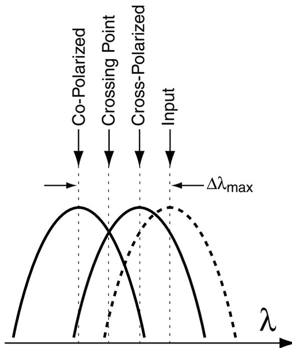
**Fig. 3.13:** Simple diagram showing the blue-shift in the probe spectrum. Two extreme cases correspond to co-polarized and cross-polarized pump and probe combinations. Intersection point is approximately in the midpoint between the two extreme cases.
