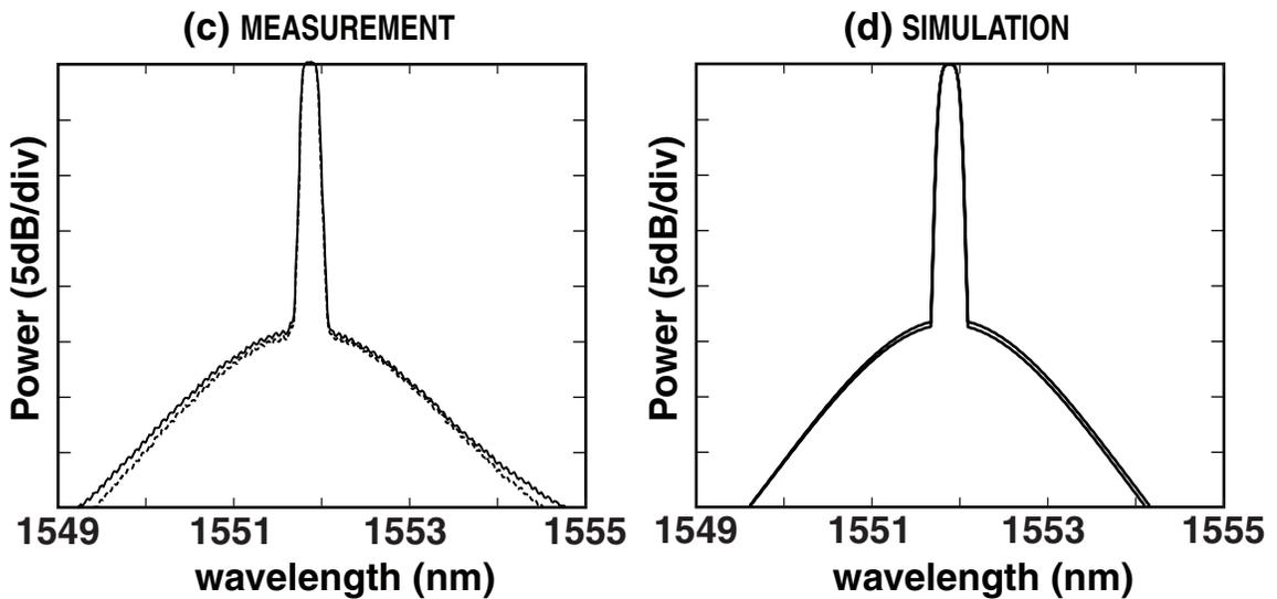
**Fig. 3.22:** Part (a) (measurement) and part (b) (simulation) plot the polarization dependence of XPM spectrum (two extreme probe polarization cases) while the pump polarization is adjusted to generate the maximum polarization dependence. Parts (c) and (d) plot the same spectra while the pump polarization state is chosen to minimize the polarization dependence.
