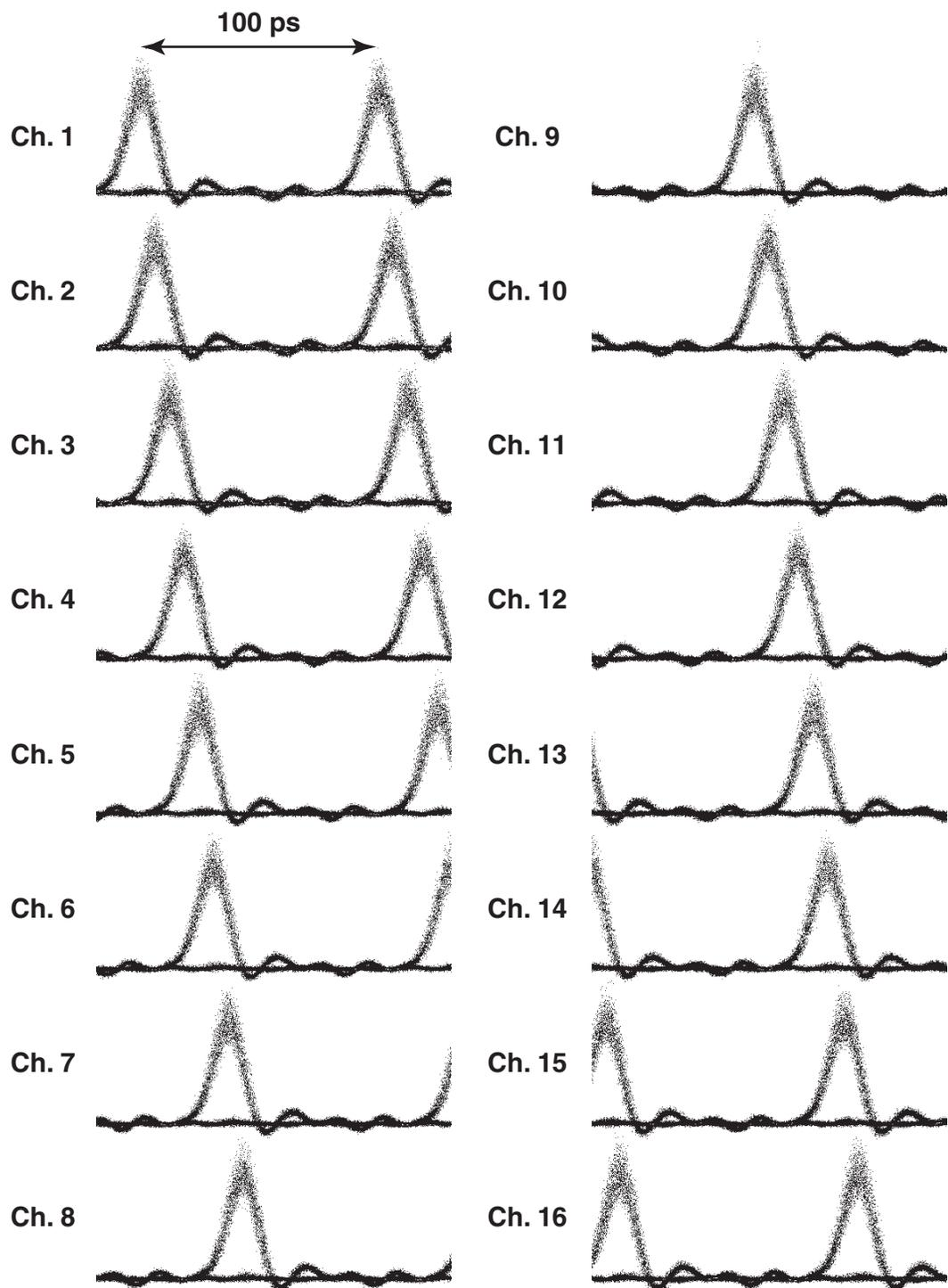
**Fig. 3.19:** Eye diagrams of the 16 channels in the 160 Gb/s data captured as the data polarization is scrambled.
