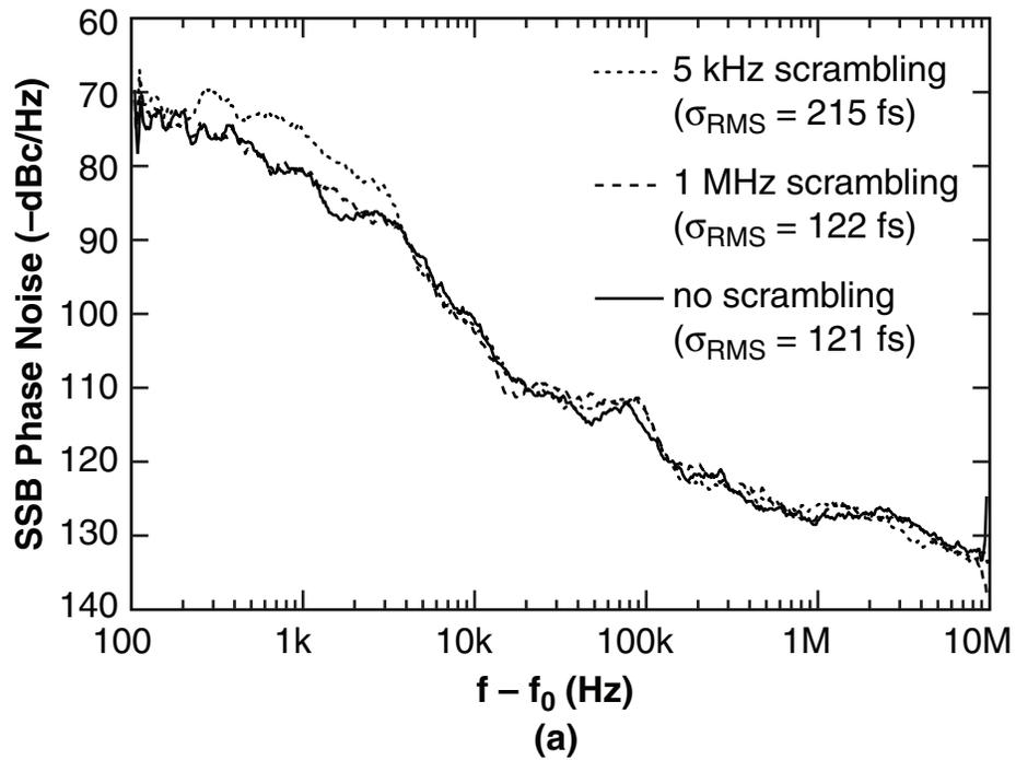
**Fig. 2.19:** Measured single-sideband phase noise of the recovered clock, when the data polarization state is scrambled at two different speeds. When the polarization fluctuations are within the PLL bandwidth, the timing jitter increases as a result of polarization-induced timing fluctuations.
