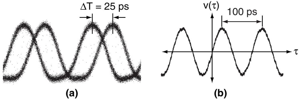
**Fig. 2.30:** (a) Measured eye diagram of the dithered clock. The dither amplitude of 25 ps is determined by the length of PM fiber. (b) The measured error signal always exhibits a zero-crossing at  $\tau = 0$ .
