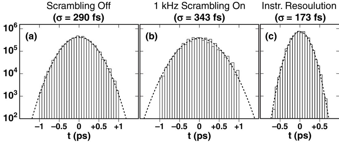
**Fig. 2.20:** Histograms showing the distribution of the zero-crossing time for the electrical clock when the oscilloscope is triggered with the original clock. Histograms show the results for: (a) without scrambling, (b) with 1 kHz scrambling and (c) intrinsic jitter measured by using the original clock instead of the recovered clock.
