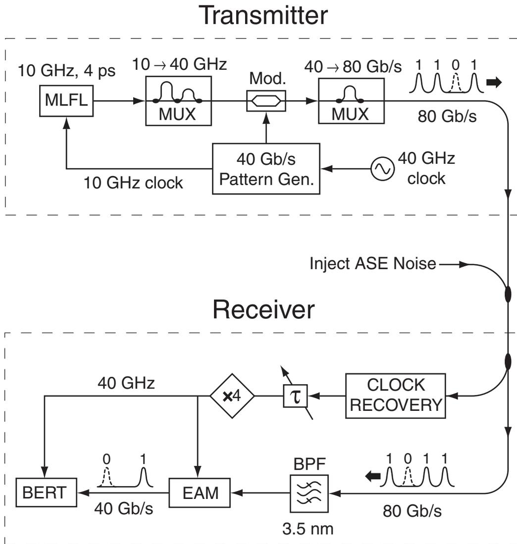
**Fig. 2.10:** Diagram of 80 Gb/s optical transmitter, demultiplexer, and receiver used to characterize the clock recovery system. Instead of varying the received optical power, the optical signal-to-noise ratio was adjusted by injecting broadband optical noise prior to the receiver.
