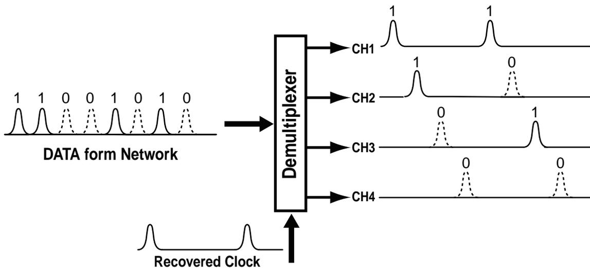
**Fig. 1.3:** Diagram of a demultiplexer in OTDM system.
