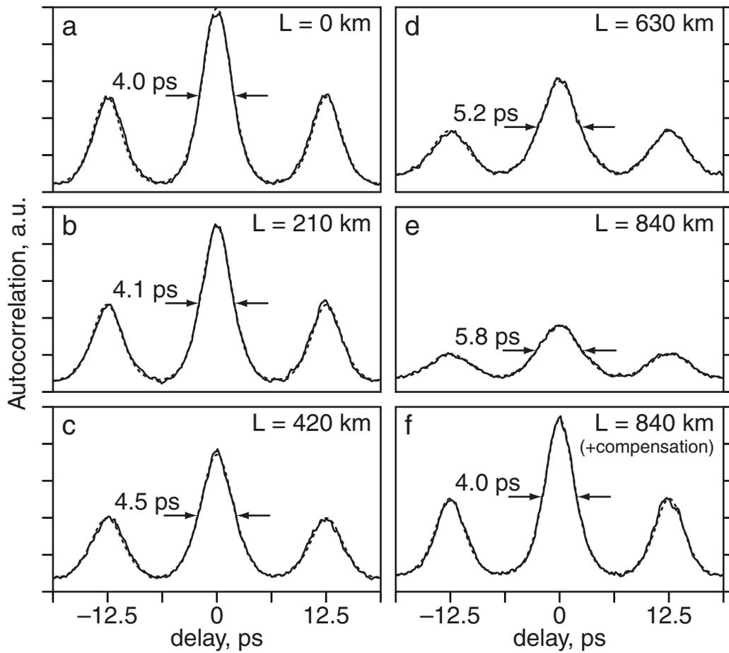
**Fig. 2.26:** Time-gated autocorrelation measurements of 80 Gbit/s data after 0, 1, 2, 3, and 4 round trips. The final trace shown in (f) depicts the autocorrelation after residual dispersion is compensated by adding 100 meters of additional fiber.
