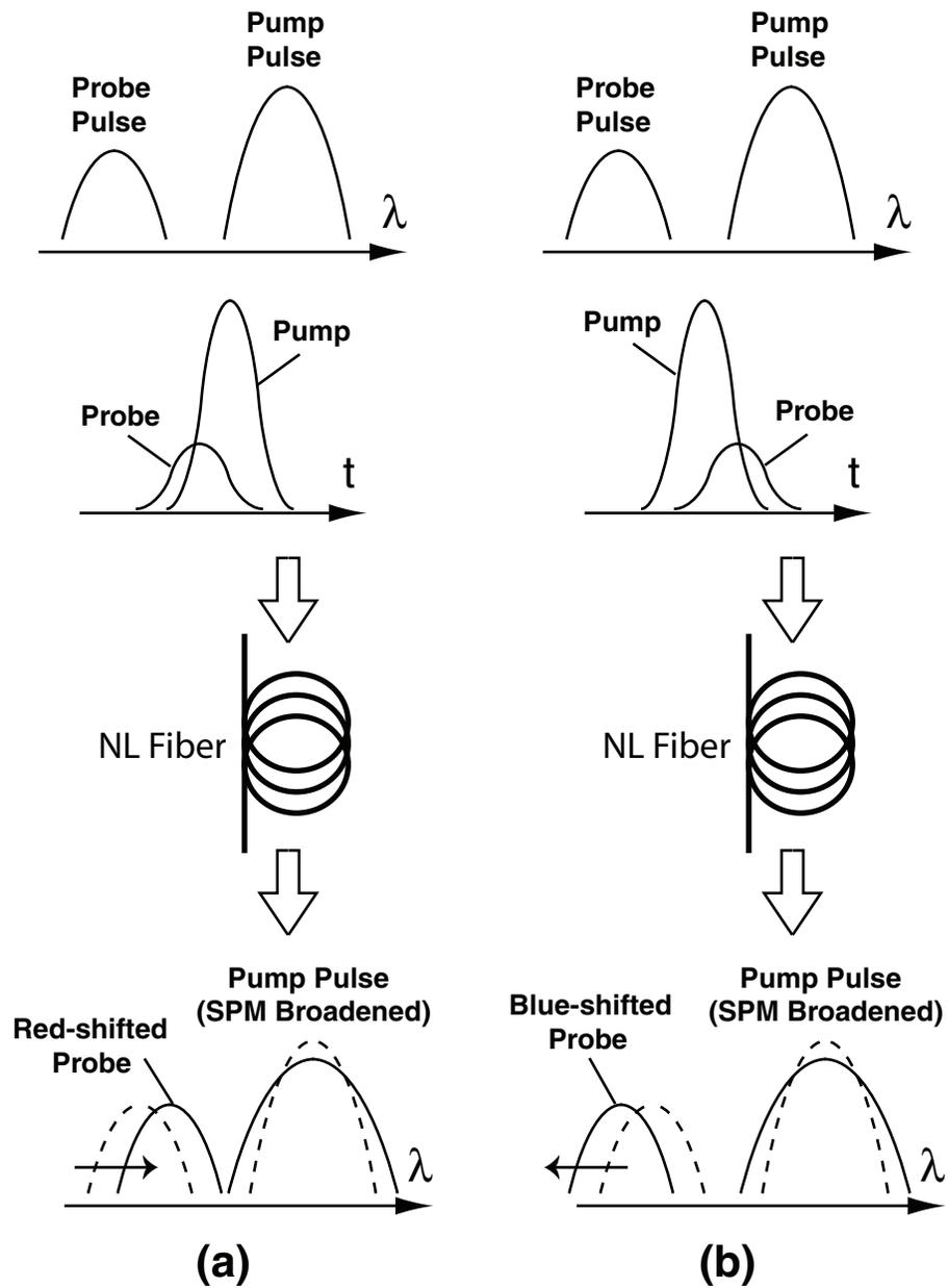
**Fig. 3.10:** Cross-phase modulation between two optical pulses. Spectral shift on the probe can occur to either blue (a) or red (b) side of the spectrum depending on the relative delay between the two pulses.
