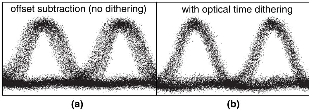
**Fig. 2.33:** Eye diagram of received 10 Gb/s data, measured while the polarization state is varied. (a) The undithered system exhibits significant polarization-dependent timing, as described in Sec. 2.4. (b) The dithering clock recovery instead locks to the peak of the cross-correlation signal, which reduces the polarization dependence.
