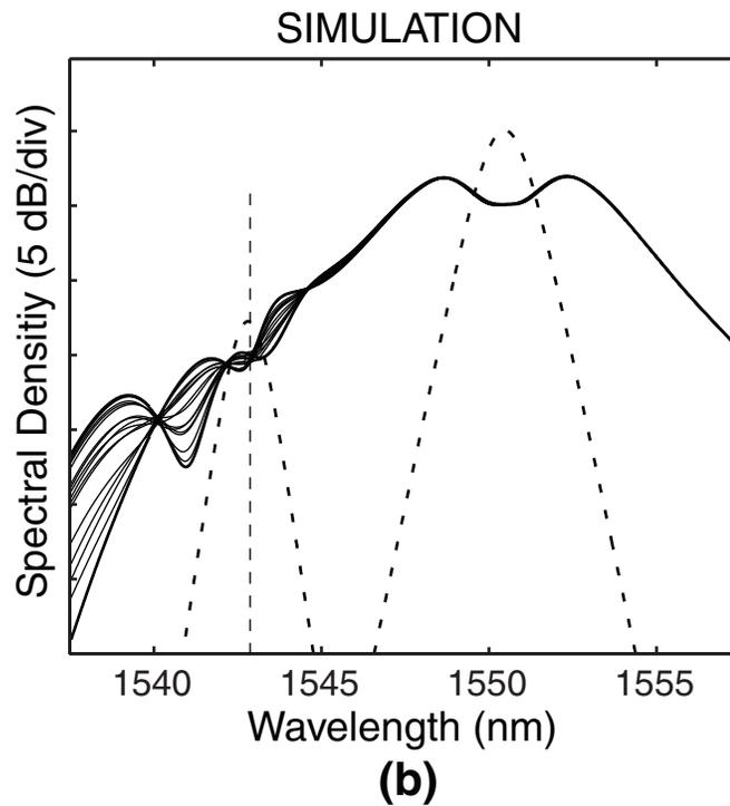
**Fig. 3.12:** Cross-phase modulation between two optical pulses. Part (a) shows the measured spectra for two extreme polarization states (solid curves) and the input spectrum (dashed curve). Part (b) plots the simulation results for the two extreme cases as well as 14 equally-spaced points on the Poincaré sphere.
