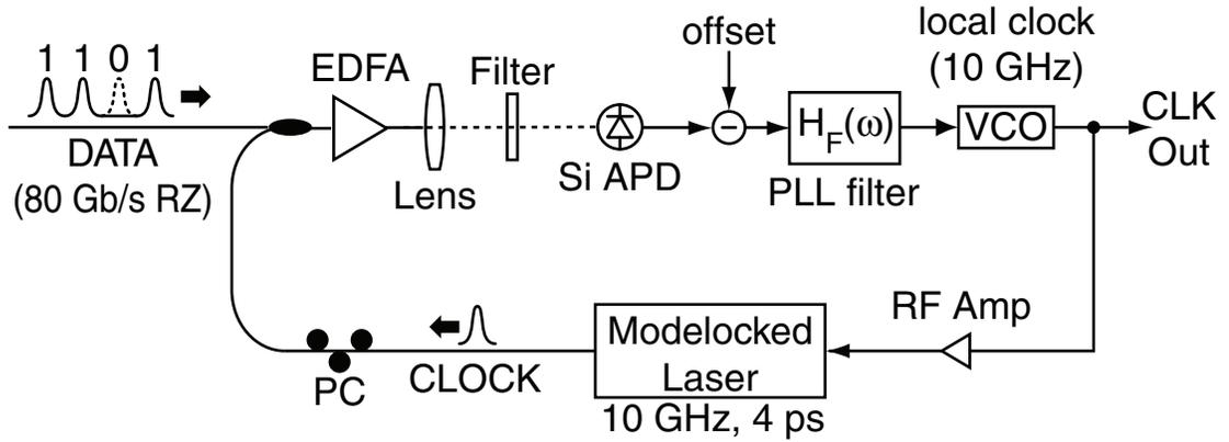
**Fig. 2.5:** Diagram of 80 Gb/s optical clock recovery system.
