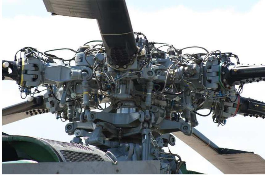
Figure 1.2: Example of swashplate with many parts (Source: [www.fightercontrol.co.uk](http://www.fightercontrol.co.uk)).
