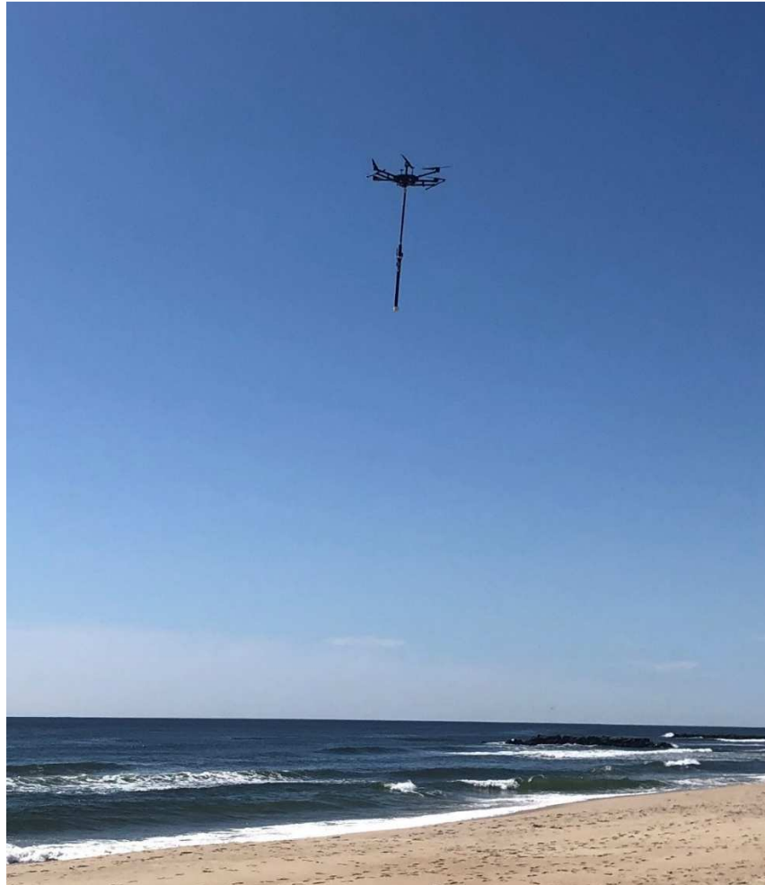
Figure 5. Matrice 600 Pro 6-rotor drone with MAGPi ML-4 on carbon fiber rod in flight. Photo by the author.
