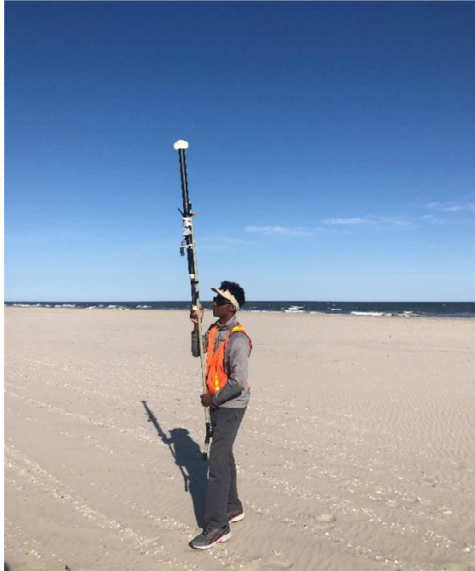
Figure 9. Handheld magnetometer data collection for the Sindia carried by an undergraduate student from West Chester University. Photo by the author.
