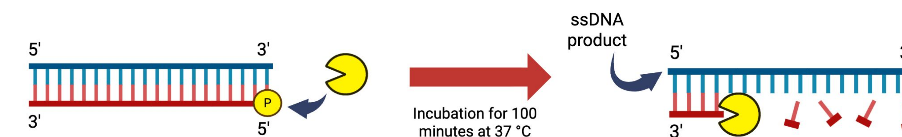
Figure 3. The lambda exonuclease enzyme is able to recognize and selectively degrade strands of dsDNA that were tagged with a 5' phosphate reverse primer during PCR.
