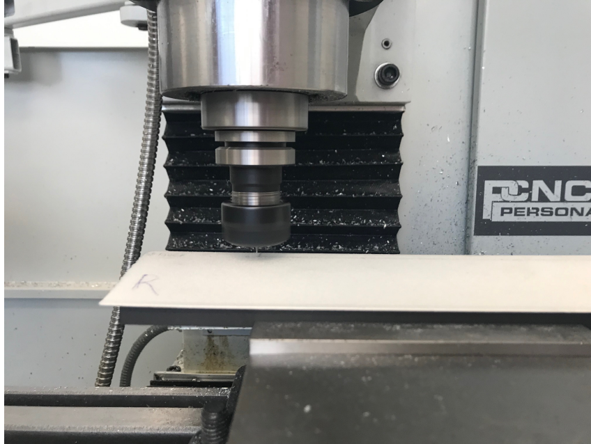
Figure 2.7: Spar cut on mill using 1/16 inch aluminum mill bit
