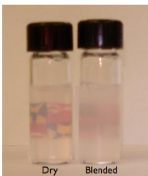
**Figure 2.7.** Solutions of cationic bare vesicles formed from 1) solid surfactants and 2) blended surfactants. The University of Maryland seal can be seen behind vesicles prepared using dry surfactants. Vesicles prepared by blended surfactants yielded significantly cloudier solutions containing larger vesicles, which scattered light to a greater degree.
