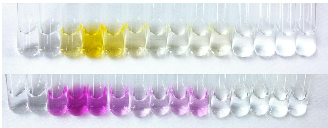
**Figure A.4.** CTAT-rich vesicles containing phenol red after SEC purification. A) All fractions are yellow in color from the monoanion at pH 7. B) After addition of NaOH, all fractions turned fuchsia in color, indicating the presence of the dianion in solution. Vesicle-containing fractions incorporated phenol red, leaving the acidic proton accessible for the acid-base reaction.
