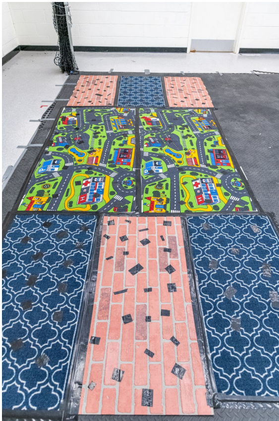
Figure B.9: Different textured carpets laid on the ground during real experiments to aid robust homography estimation from EVHomographyNet.
