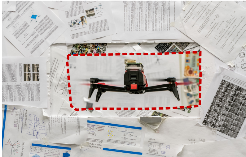
Figure A.14: Quadrotor traversing an unknown window with a minimum tolerance of just 5cm. (red dashed line denotes C .)
