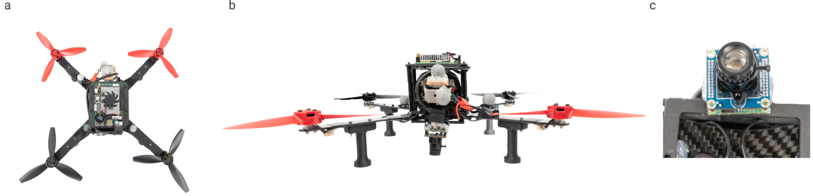
Figure F.3: PRG Husky-360 \gamma platform used in flight experiments. (a) Top view, (b) front view, (c) down-facing leopard imaging camera.
