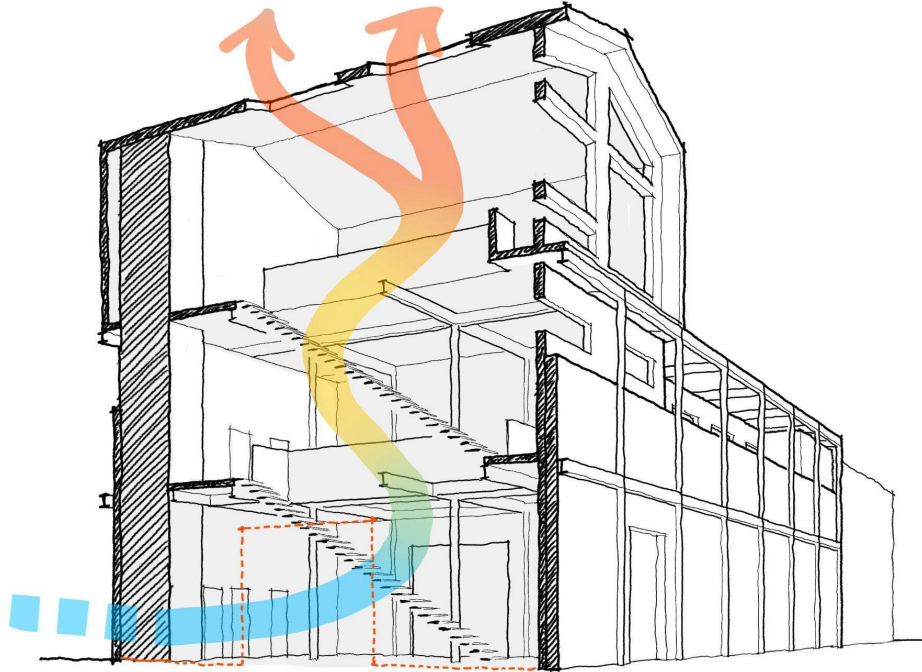
Fig. 55: Author's own. Climate strategies diagram showing passive ventilation via the skylights and existing side door.
