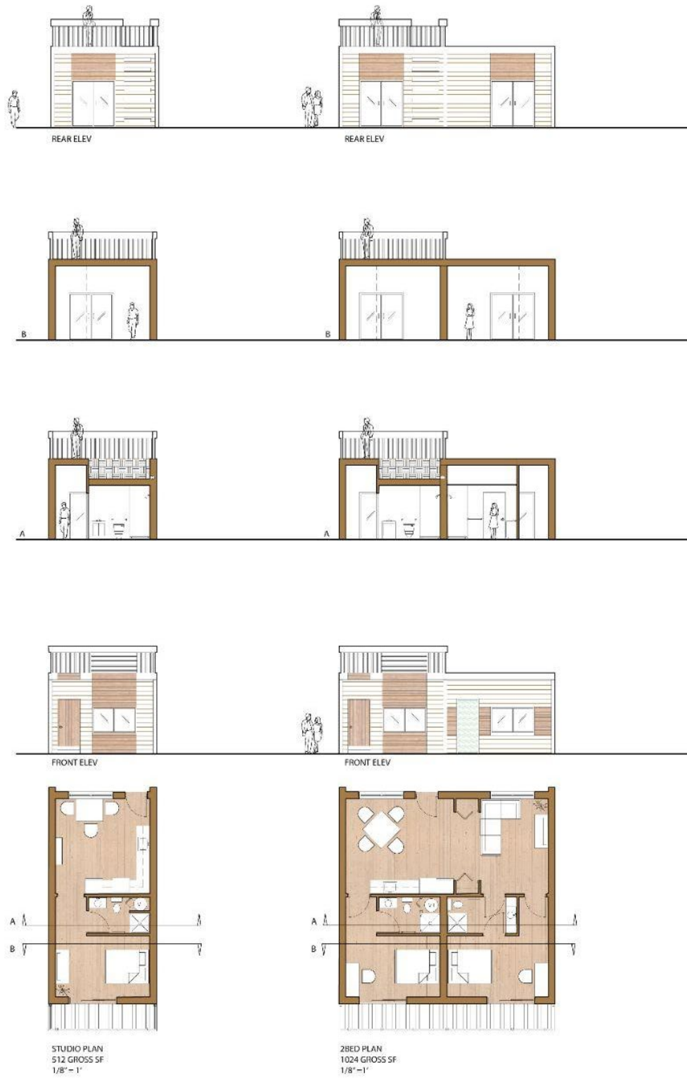
Fig. 59: Author's own. Plans, sections, elevations for the timber housing module, both sizes.
