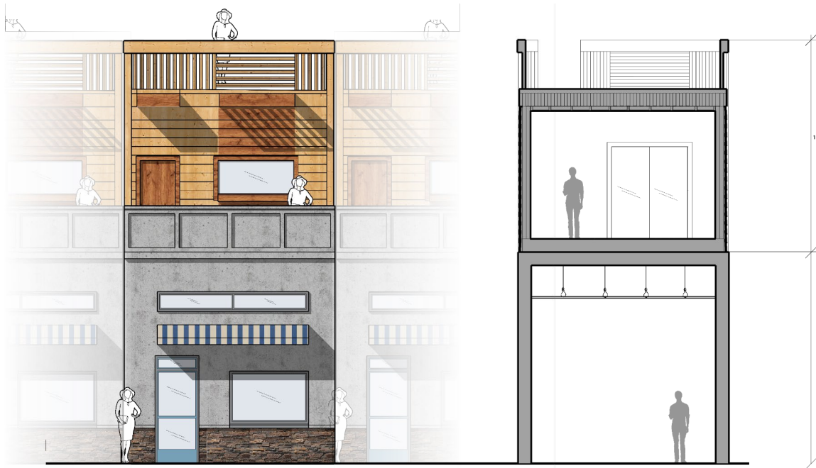
Fig. 58: Author's own. Front elevation and transverse section of the timber module and concrete base.
