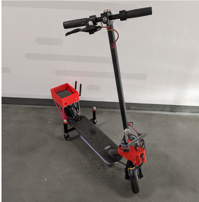
Figure 3.4: Peter Parker, our third and latest prototype autonomous e-scooter. Peter is still under development and not yet operational.
