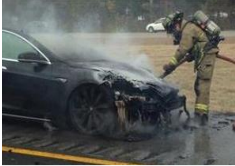
Figure 3-2 Thermal Failure in Tesla Model S Battery Pack [50]
