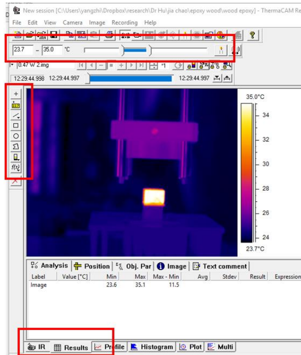
Figure 0-6 Screenshot of ThermoCAM Software Control Interface
