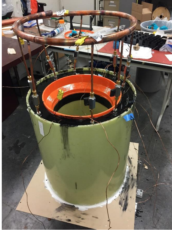
Figure 4-12 Digital Picture of Final Magnetic Field Wire Housing after Epoxy Potting
