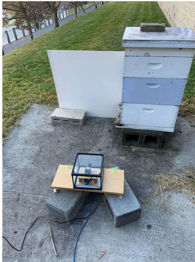
Fig. 7. A demonstration of the setup of the DVS in front of the hive. The white poster board was used to provide a uniform, high-contrast background. The DVS is enclosed in a glass box to allow long-term recordings without concerns about weather damage. The box was tested to ensure that glare and condensation would not have an impact on its performance.
