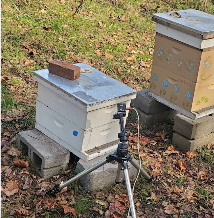
Fig. 4. The image above depicts early proof of concept tests with the DVS 128 at hives owned by the University of Maryland's beekeeping club. The low-resolution sensor had to be very close to the hive to detect bees.
