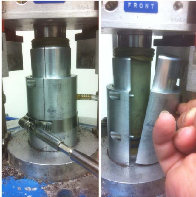
Figure 5.5 Removal of Split Mold
