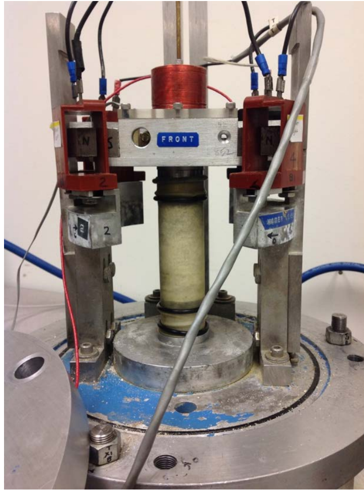
Figure 5.6 Sand Column before testing
