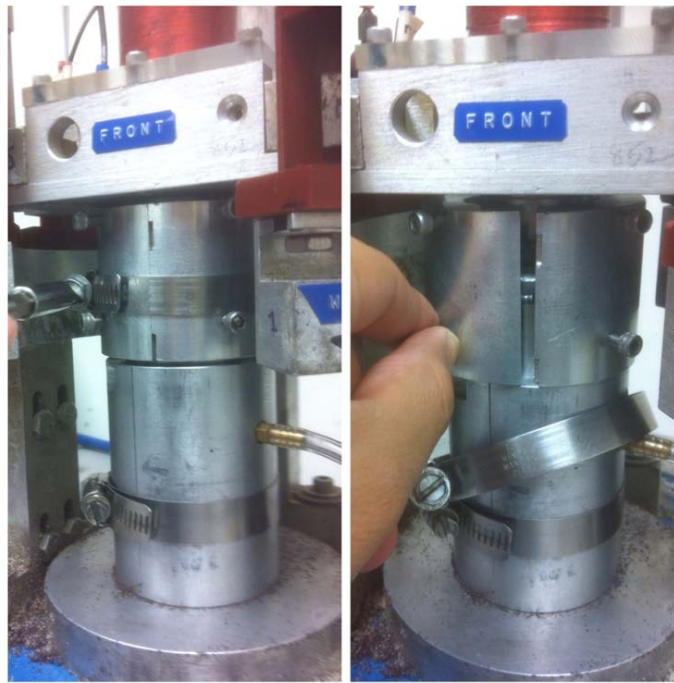
Figure 5.4 Removal of Split Top Collar
