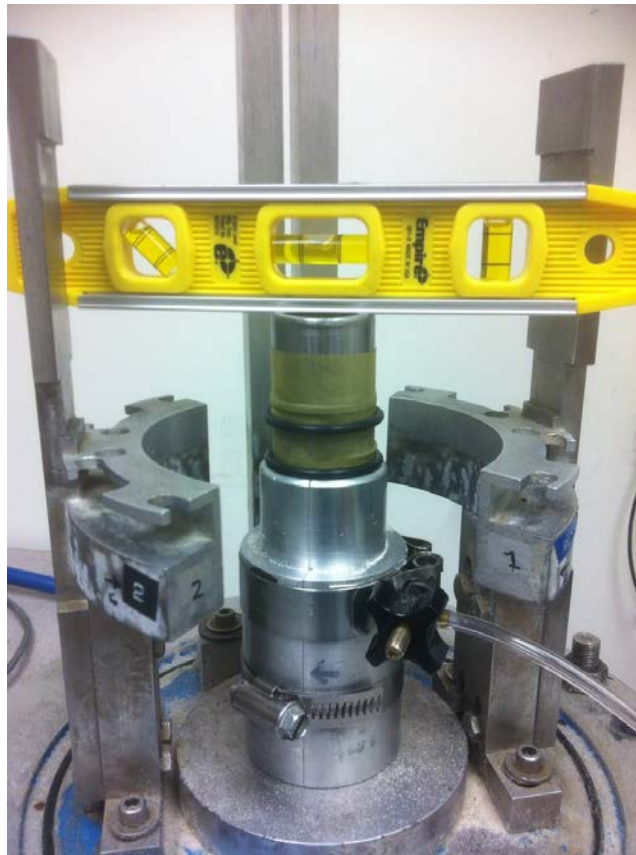
Figure 5.2 Bulb leveler on top of sand column during preparation of the sample
