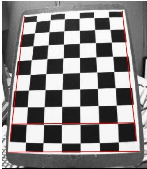
Figure 5: Example of Radial Distortion, by OpenCV ( https://docs.opencv.org/4.x/dc/dbb/tutorial_py_calibration.html )
