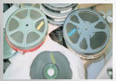
Films with A-D strips, to detect and measure film deterioration
