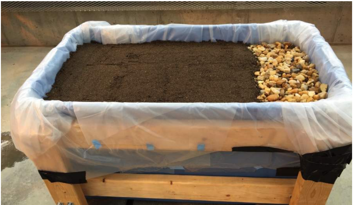
Figure 2-3: Completed Mesocosm Side and Top Views. (Top) Side view of 30% Dickerson wetland mesocosm setup with bedding thicknesses. Bedding thicknesses not drawn to scale. (Bottom) Top view of 30% Dickerson wetland mesocosm setup prior to planting. Seen at right is the gravel inlet structure.
