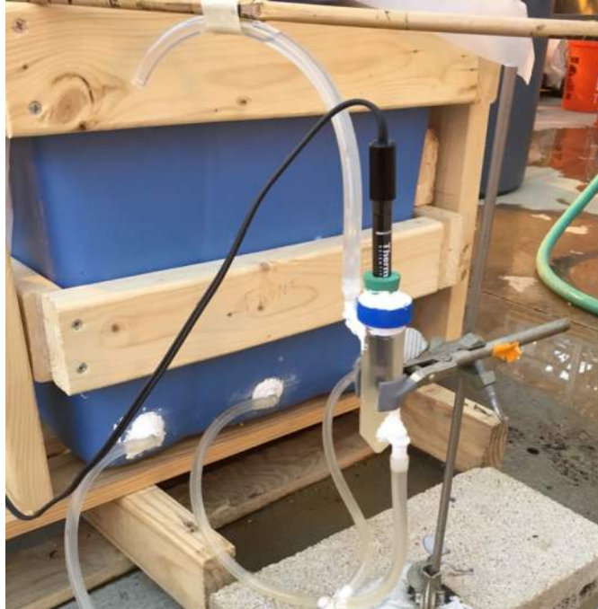
Figure 2-4: Mesocosm Front View. Front view of effluent ports with ORP electrode setup on 15% Dickerson wetland mesocosm.
