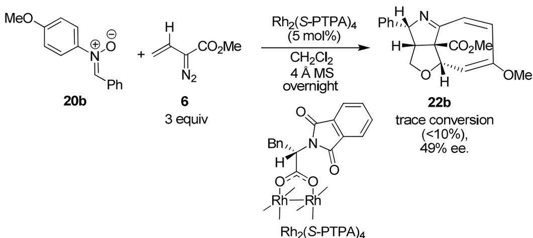
**Scheme 3.21**  $\text{Rh}_2(\text{S-PTPA})_4$ -catalyzed Cascade Reaction of **20b**.
