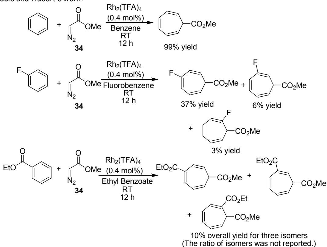
**Scheme 3.13** Buchner Reactions of **34** with Benzene, Fluorobenzene and Ethyl Benzoate Catalyzed by  $\text{Rh}_2(\text{TFA})_4$  (yields were determined by gas chromatography).
