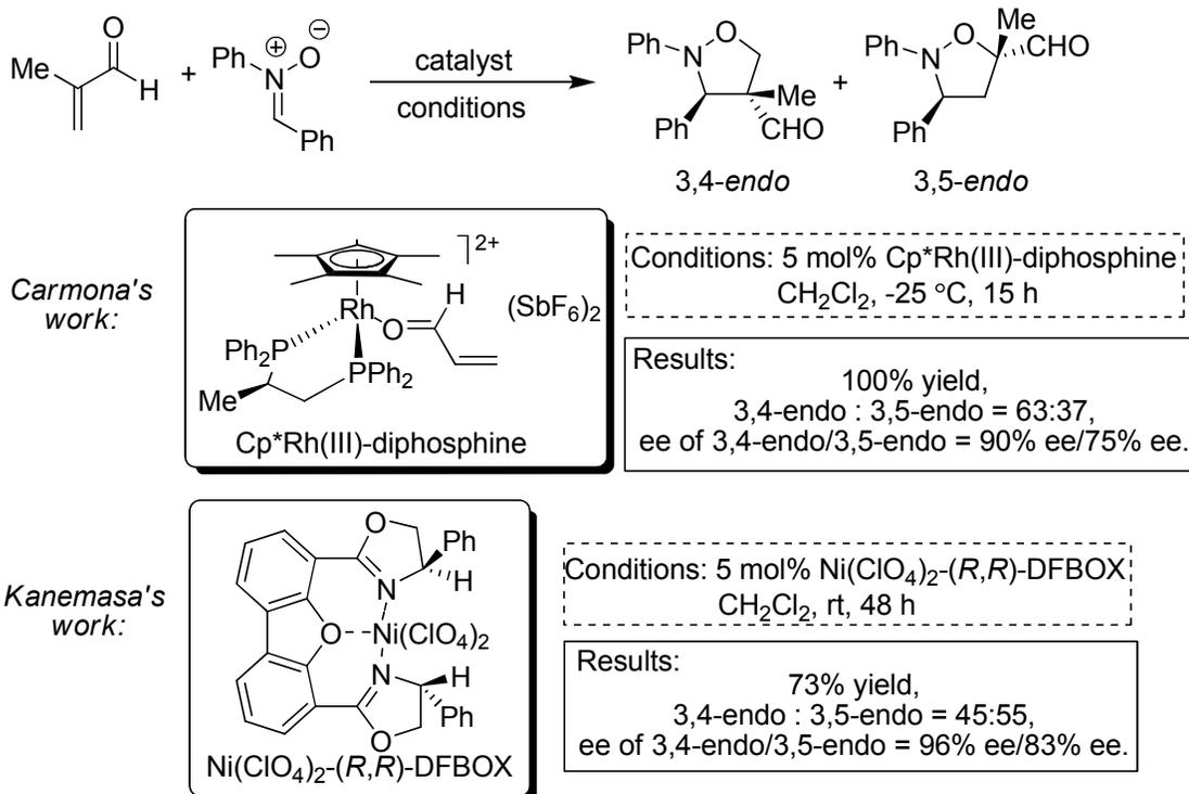
**Scheme 1.12** Carmona's Rh(III) catalyst and Kanemasa's Ni(II) catalyst in the Dipolar Cycloaddition Reaction of *N*, $\alpha$ -Diphenylnitrone with Methacrolein.
