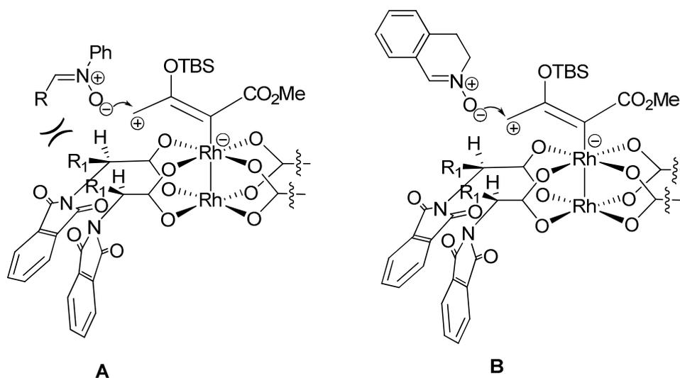
**Figure 2.5** Approaching Modes of an Acyclic Nitron (**A**) and a Cyclic Nitron (**B**) to the Rhodium Vinylcarbene from **42**.
