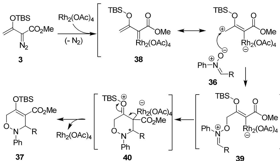
**Scheme 2.26** Mechanism of the [3+3]-Cycloaddition Reaction of the Siloxyvinyl diazoacetate **3** and the Nitron **36** Catalyzed by Rhodium Acetate.
