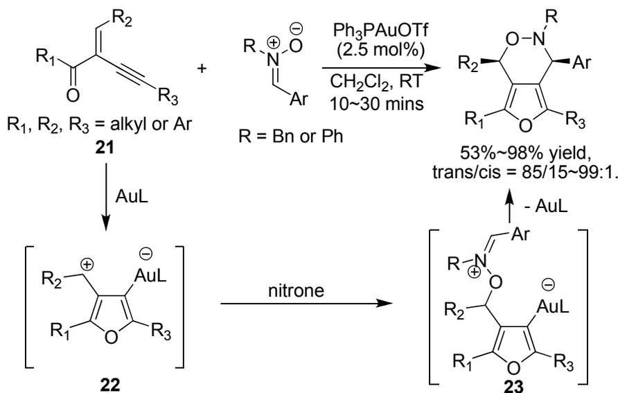
**Scheme 2.17** Gold Catalyzed [3+3]-Cycloaddition Reactions of 2-(1-Alkynyl)-2-alken-1-ones with Nitrones.
