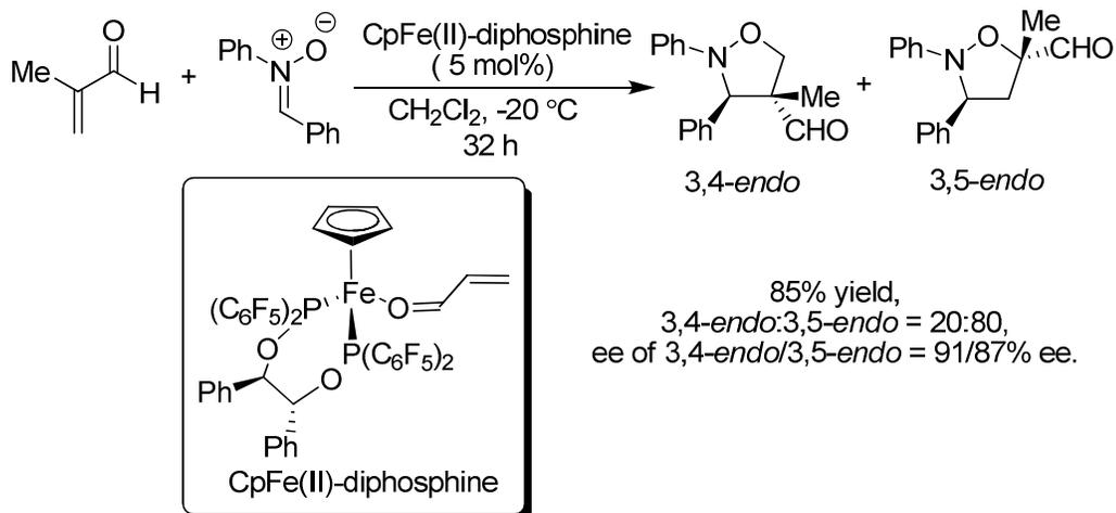
**Scheme 1.10** CpFe(II)-diphosphine Catalyzed Cycloaddition Reaction of *N*, $\alpha$ -Diphenylnitrone with Methacrolein.
