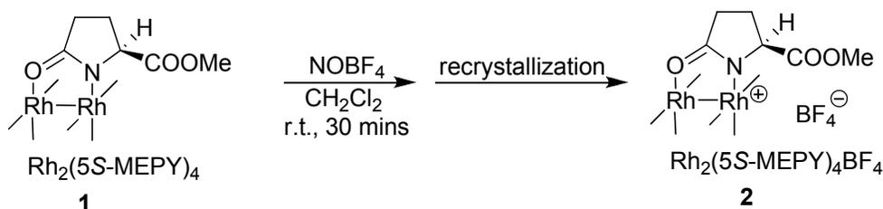
Note: NOSbF<sub>6</sub> can be used instead of NOBF<sub>4</sub> and then Rh<sub>2</sub>(5S-MEPY)<sub>4</sub>SbF<sub>6</sub> will be formed.
