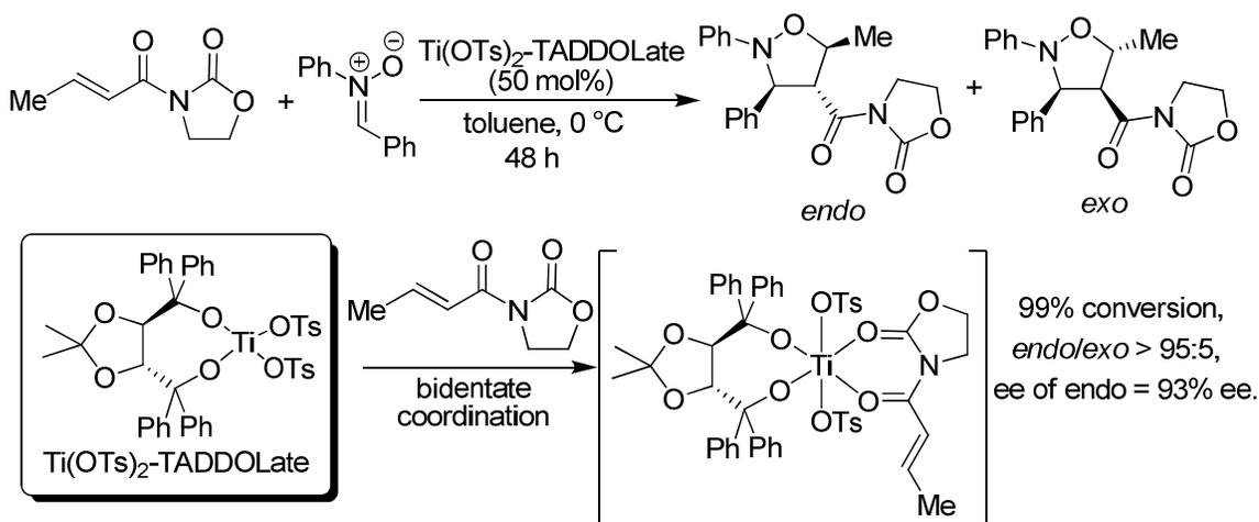
**Scheme 1.8**  $\text{Ti}(\text{OTs})_2$ -TADDOLate Catalyzed Dipolar Cycloaddition Reaction of *N*, $\alpha$ -Diphenylnitrone with the Dipolarophile Functionalized by Oxazolidinone.
