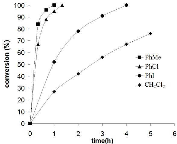
**Figure 1.5** Plot of Conversion (%) as a Function of Time for the Standard Reaction of *N*, $\alpha$ -Diphenylnitrone with Acrolein Catalyzed by  $[\text{Rh}_2(5S,R\text{-MenPy})_4]\text{SbF}_6$  in PhMe, PhCl, PhI, and  $\text{CH}_2\text{Cl}_2$  at 0 °C.
