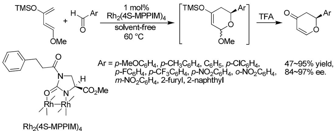
**Scheme 1.3** Rh<sub>2</sub>(4S-MPPIM)<sub>4</sub>-Catalyzed Hetero-Diels-Alder Reactions of Aldehydes with trans-1-Methoxy-3-(Trimethylsilyloxy)-1,3-Butadiene.
