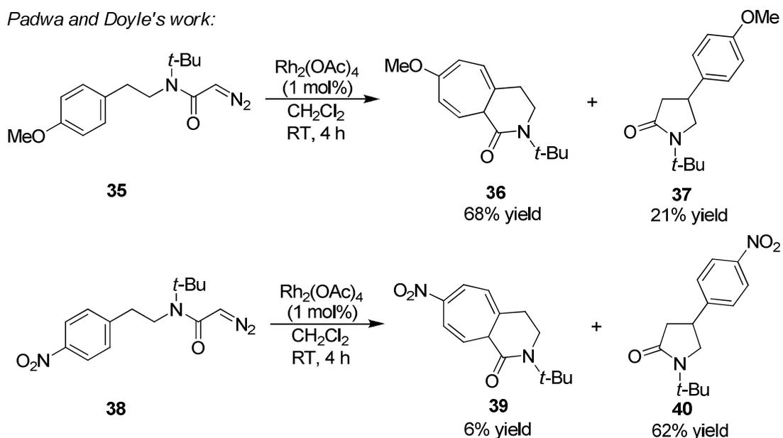
**Scheme 3.14** Yields of Intramolecular Buchner Reactions Influenced by the Electronic Properties of Aromatic Rings.
