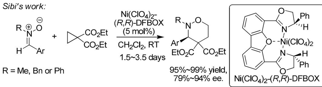
**Scheme 2.15** Chiral Lewis Acid-Catalyzed Asymmetric [3+3]-Cycloaddition Reactions of Nitrones with Cyclopropanes.
