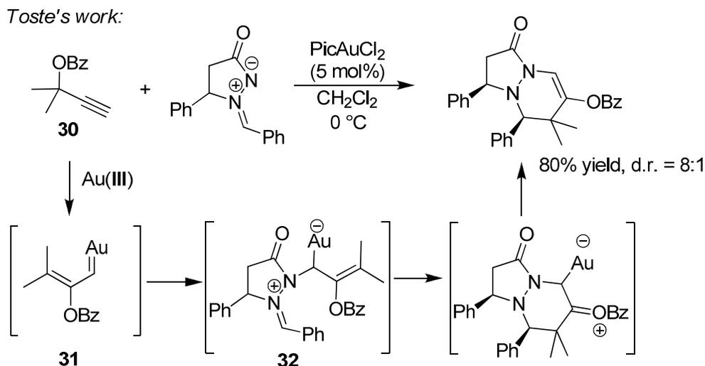
**Scheme 2.20** Gold(III)-Catalyzed [3+3]-Cycloaddition Reaction between a Propargyl Ester and an Azomethine Imine.
