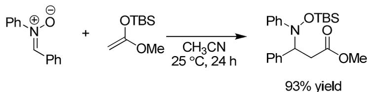
**Scheme 2.12** Nucleophilic Addition of a Silyl Ketene Acetal to *N*, $\alpha$ -diphenylnitron.
