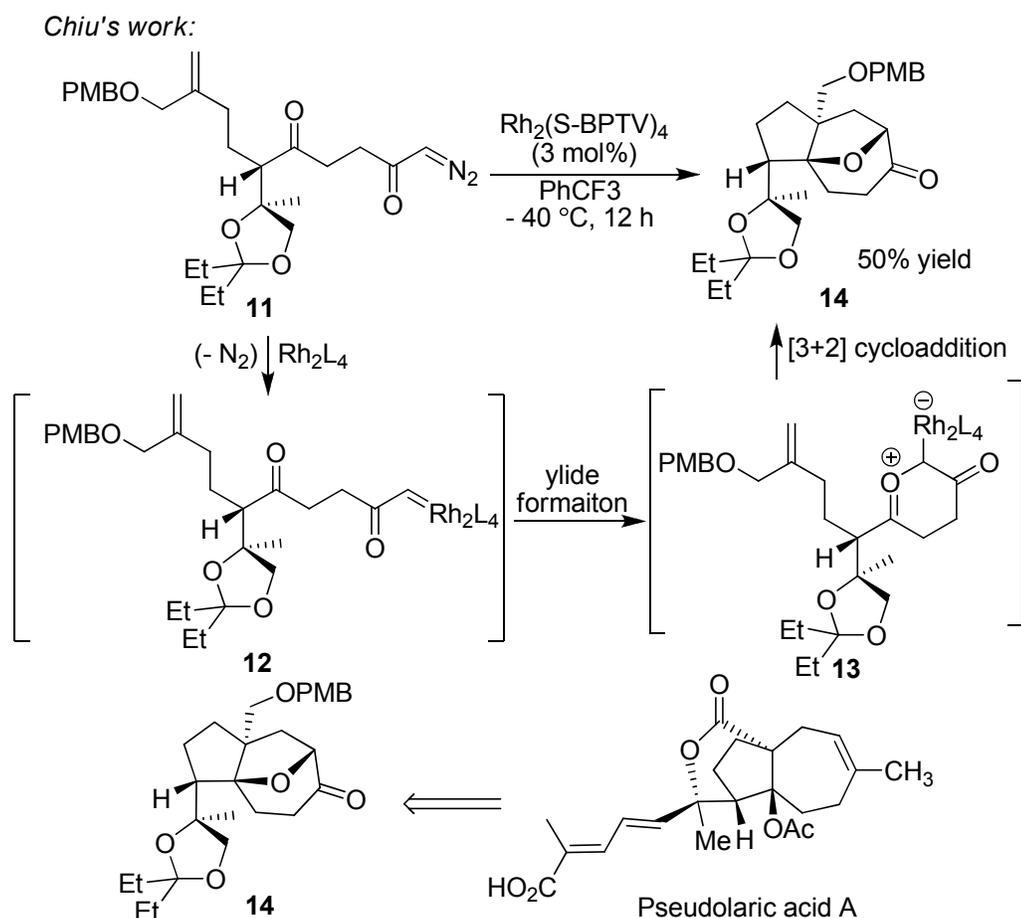
**Scheme 3.5** Intramolecular Carbonyl Ylide Cycloaddition with Alkene as the Key Step in the Total Synthesis of Pseudolaric Acid A.
