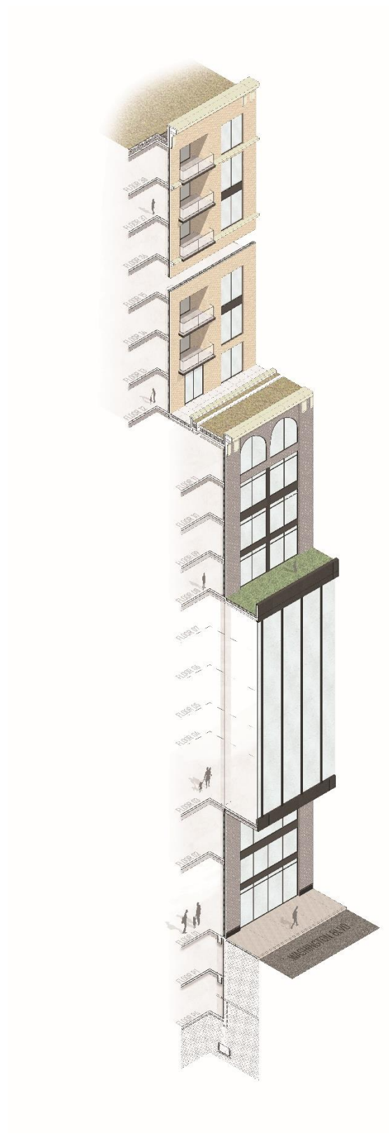
Figure 61: Isometric Wall Section Elevation (Source: J. Chase Edwards, 2023)
