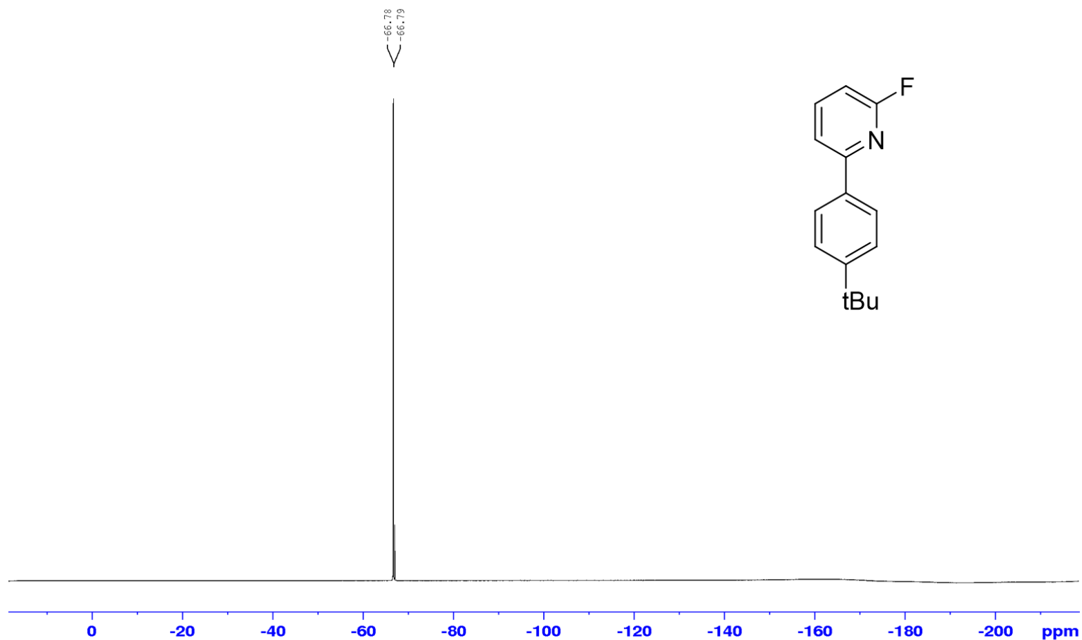
Figure S4.77. ^{19}\text{F} -NMR for 2-fluoro-6-(4- tert -butylphenyl) pyridine, 4.5-tBu in \text{CDCl}_3
