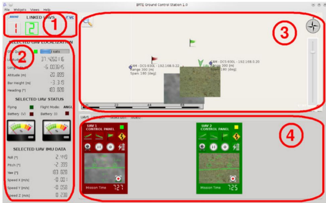
Figure 2: [36] Ground control station. (1) UAV selection, (2) Vehicle information, (3) Map display, (4) Other widgets
