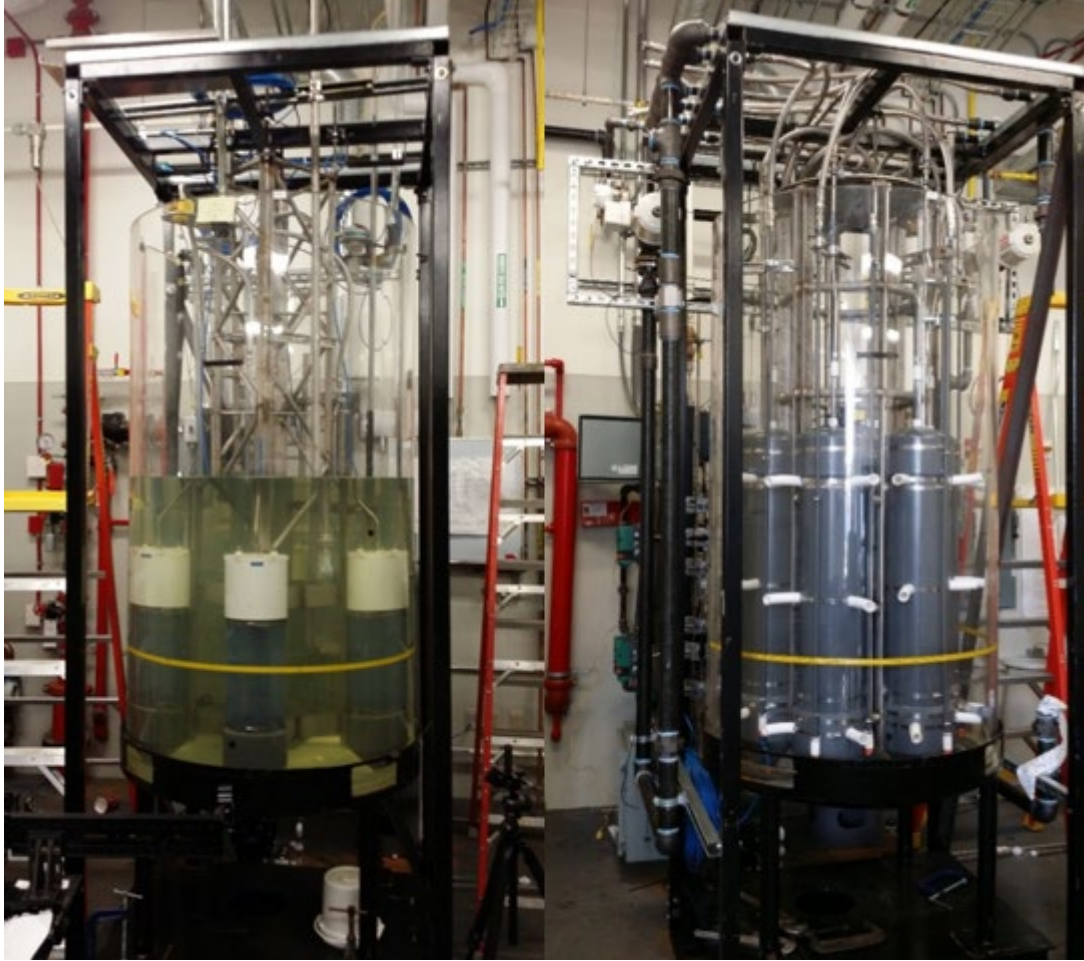
Figure 5. 1-m Diameter (left) which contains 4 PJMs and 1.2-m Diameter (right) which contains 6 PJMs (images excerpted from [7]).
