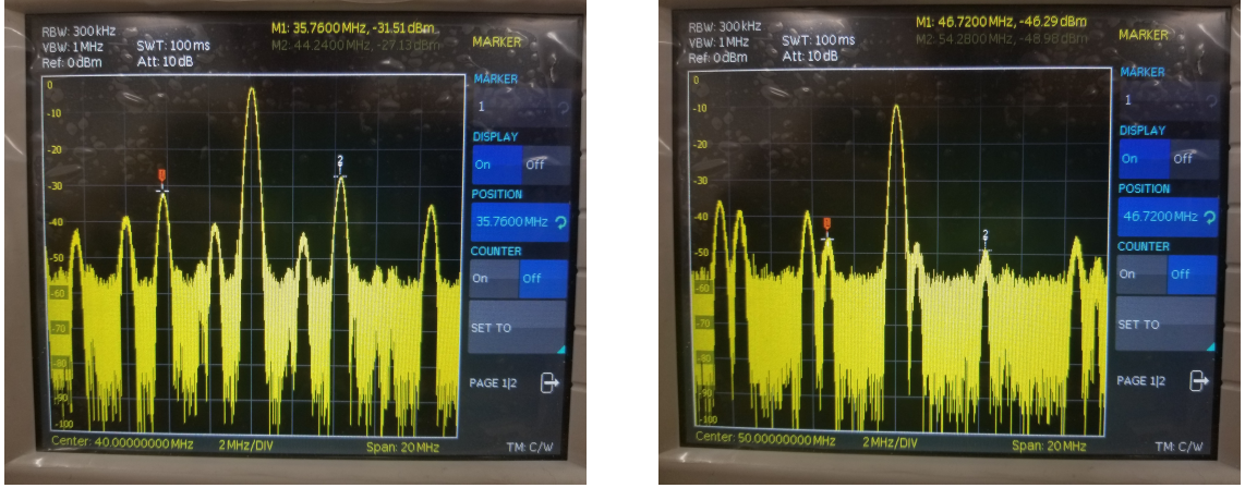
Figure 7.5: (a) Spectrum analyzer view for the mixer's output at f_{RF}=40\text{MHz} , f_{LO}=4.3\text{MHz} . (on left) (b) Spectrum analyzer view for the mixer's output at f_{RF}=50\text{MHz} , f_{LO}=4.3\text{MHz} . (on right)
