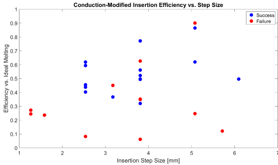
Figure 48: Conduction-corrected efficiency vs insertion step size of all insertion tests using measured internal conduction rates.
