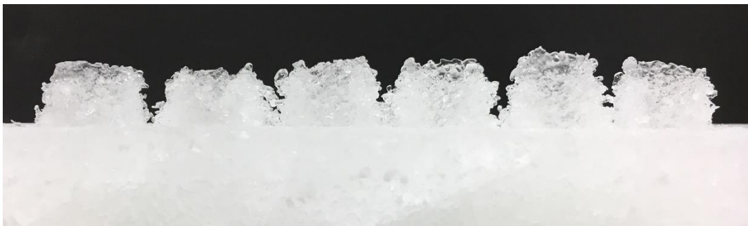
Figure 37: Formation lip shown for multiple tests on the same ice block.
