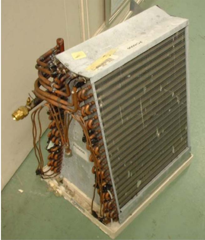
Figure 3.5 An A Type Indoor Coil
