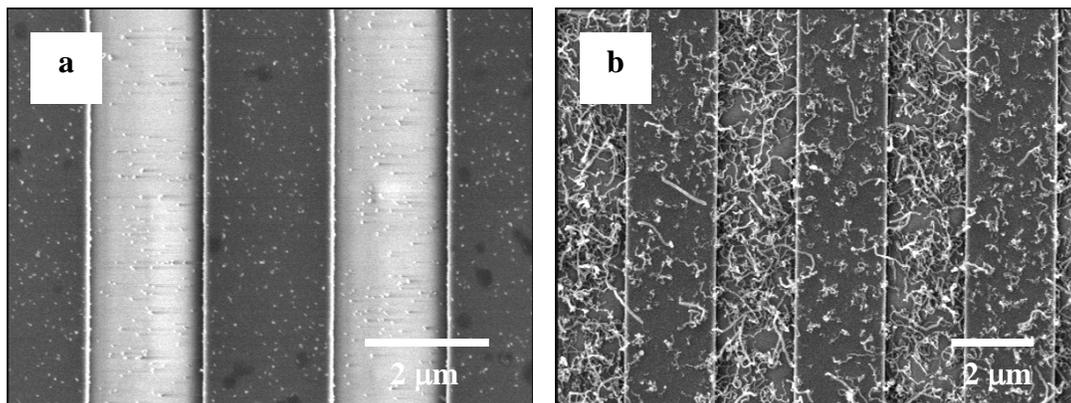
**Figure 2.5** – SEM images of microhotplate surface following (a) 30 nm sized Ni nanoparticle deposition; (b) carbon nanotube growth
