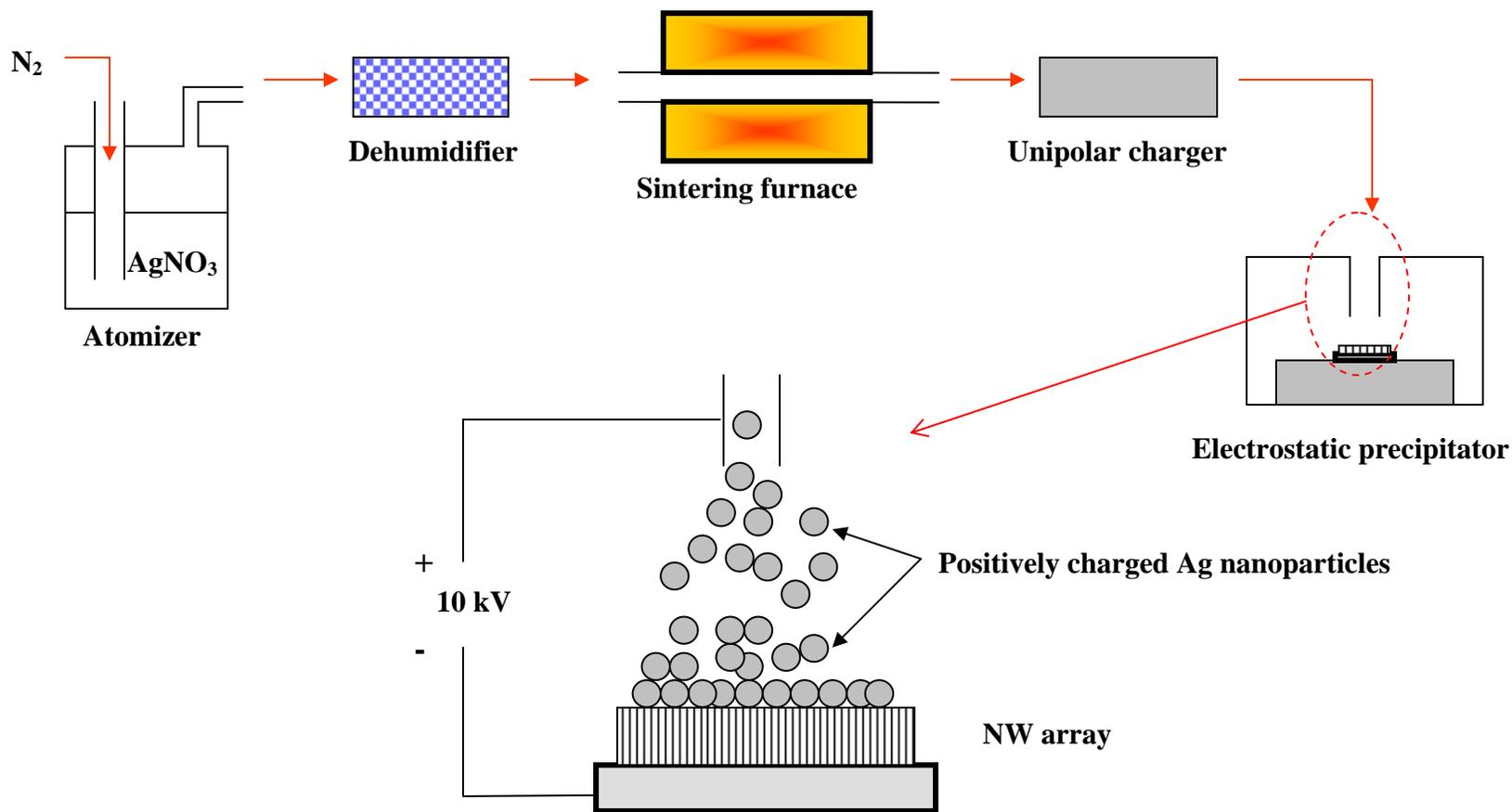
**Figure 4.8** – Schematic diagram of Ag nanoparticle generation by aerosol spray-pyrolysis followed by sintering, charging and deposition on a ZnO nanowire array within an electrostatic precipitator
