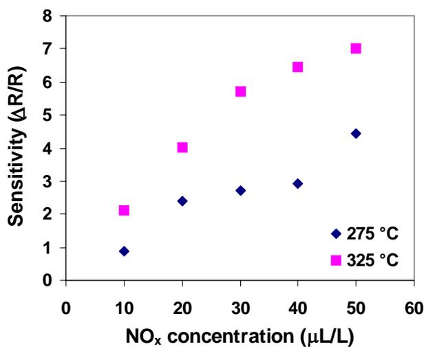
**Figure 4.18** – Sensitivity of the nanowire array to nitrous oxide, evaluated at 275 and 325 °C.
