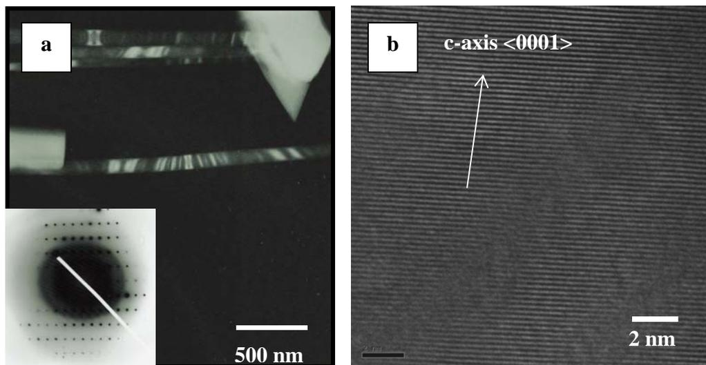
**Figure 4.5** – (a) Low-resolution TEM images of individual ZnO nanowires; Inset depicts SAED patterns from a nanowire. (b) High-resolution image of ZnO nanowire lattice planes.
