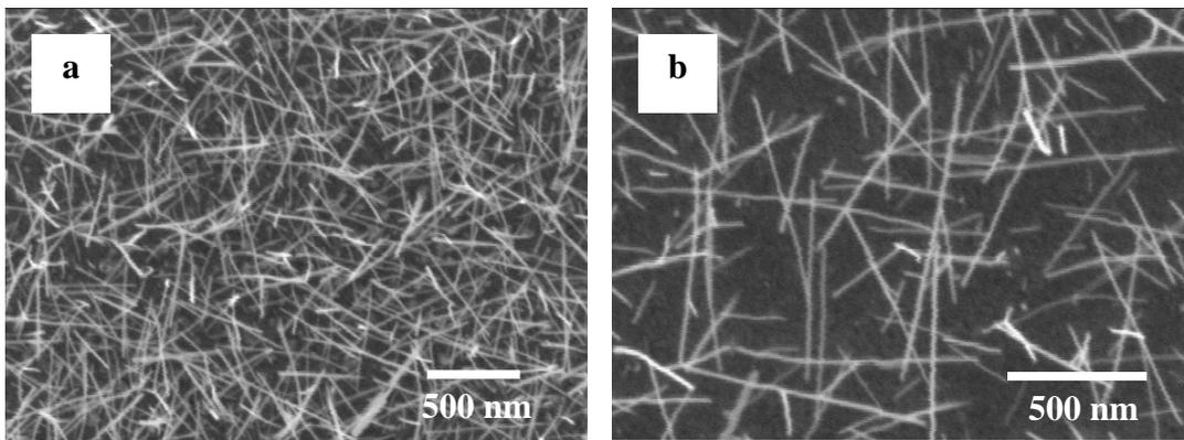
**Figure 3.4** – Uniform network of nanowires grown by heating a tungsten film at 550 °C in RF Ar/H<sub>2</sub> plasma.
