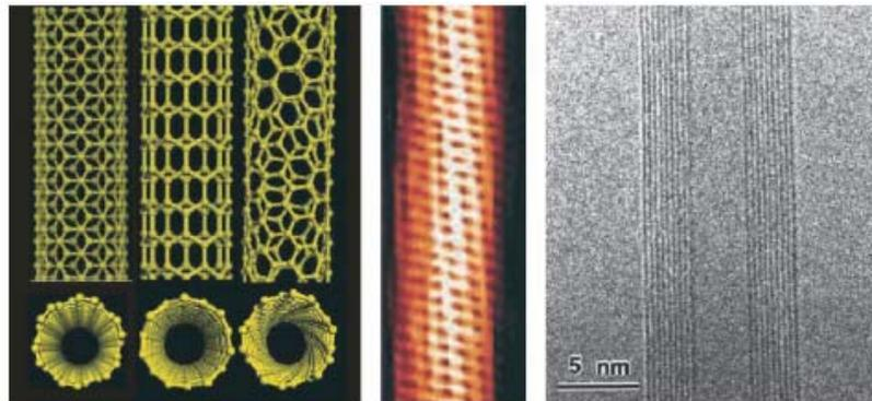
**Figure 2.1** – Schematic diagram of graphitic sheet structure of carbon nanotubes and a transmission electron microscope image of a multi-walled nanotube. Reproduced from Ref. [35].
