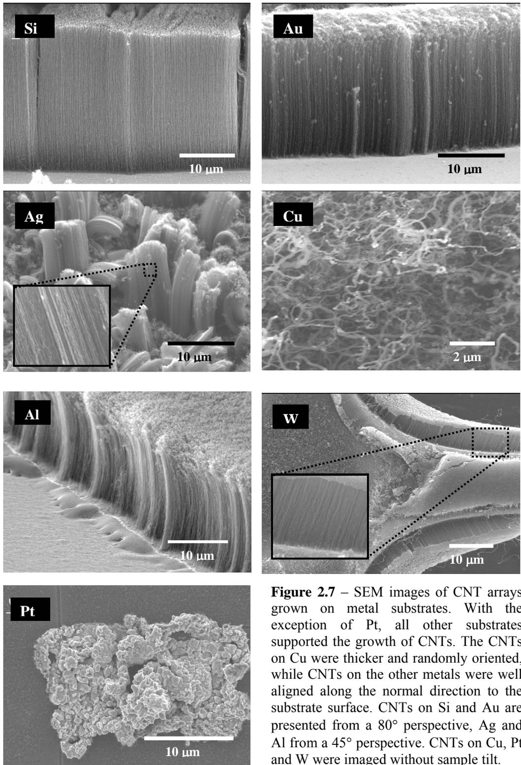
**Figure 2.7** – SEM images of CNT arrays grown on metal substrates. With the exception of Pt, all other substrates supported the growth of CNTs. The CNTs on Cu were thicker and randomly oriented, while CNTs on the other metals were well aligned along the normal direction to the substrate surface. CNTs on Si and Au are presented from a 80° perspective, Ag and Al from a 45° perspective. CNTs on Cu, Pt and W were imaged without sample tilt.
