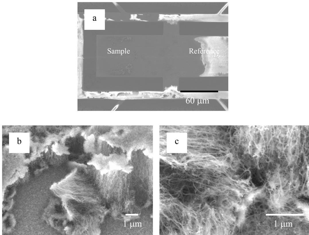
**Figure A2** – SEM images of CNTs grown on a micro-calorimeter device. (b) and (c) represent CNT forests grown on the sample zone.
