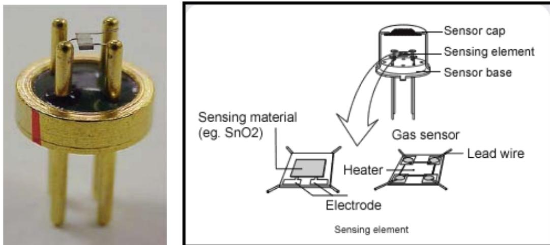
**Figure 1.3** – Digital photograph and schematic view of the components of a commercial Taguchi sensor. Reproduced from Ref [11].
