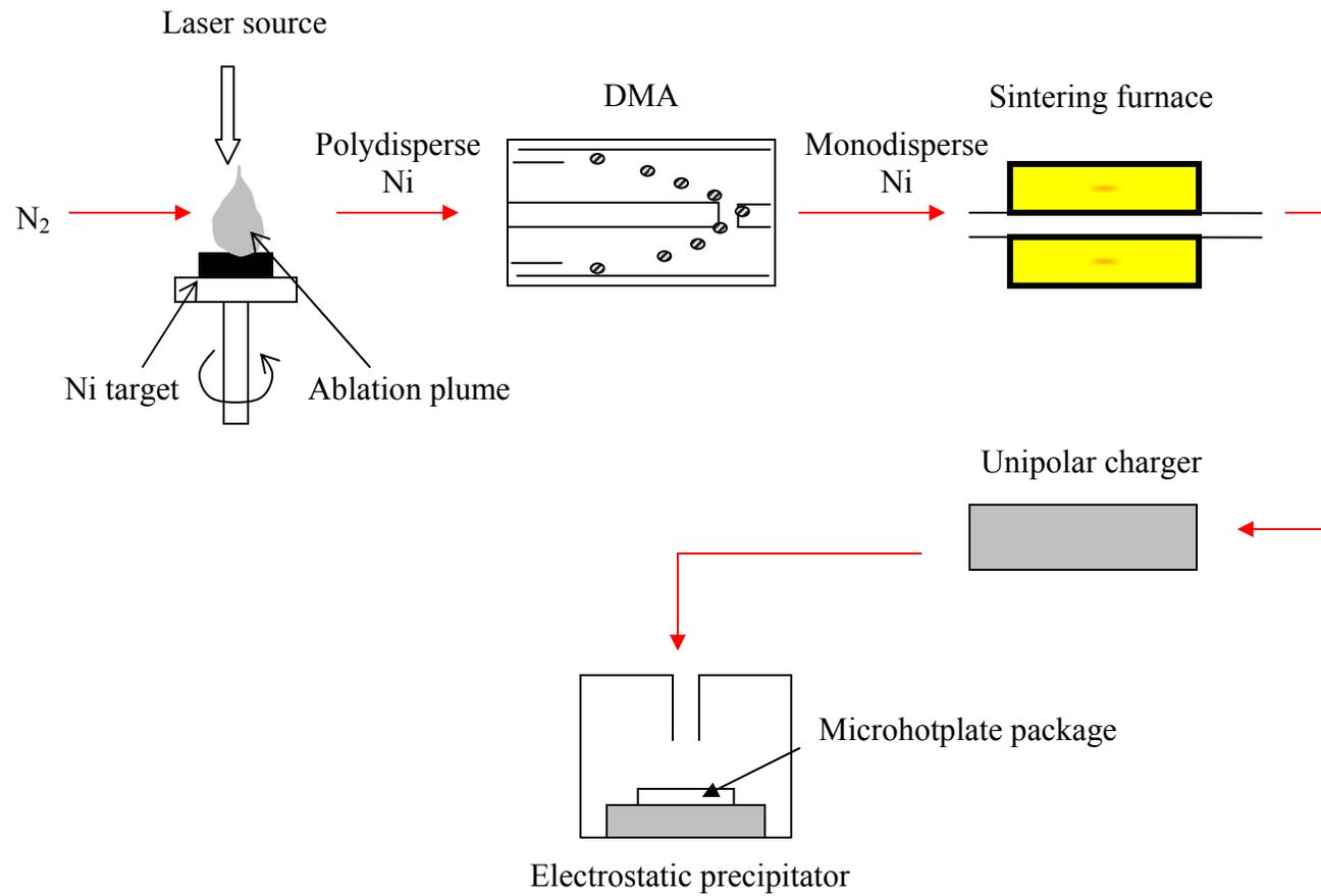
**Figure 2.4** – Schematic diagram of Ni nanoparticle generation and deposition
