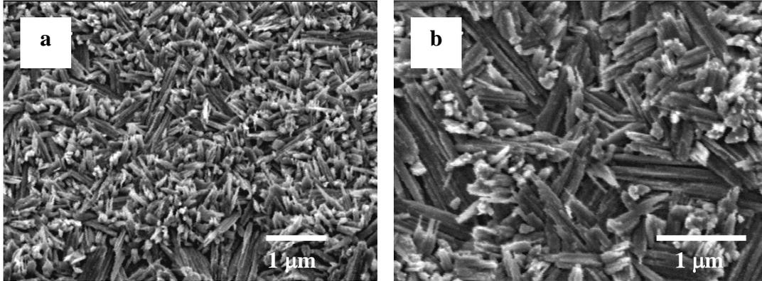
**Figure 3.3** – SEM images of grainy, nodular surface of tungsten film heat treated at 750 °C in pure Ar.
