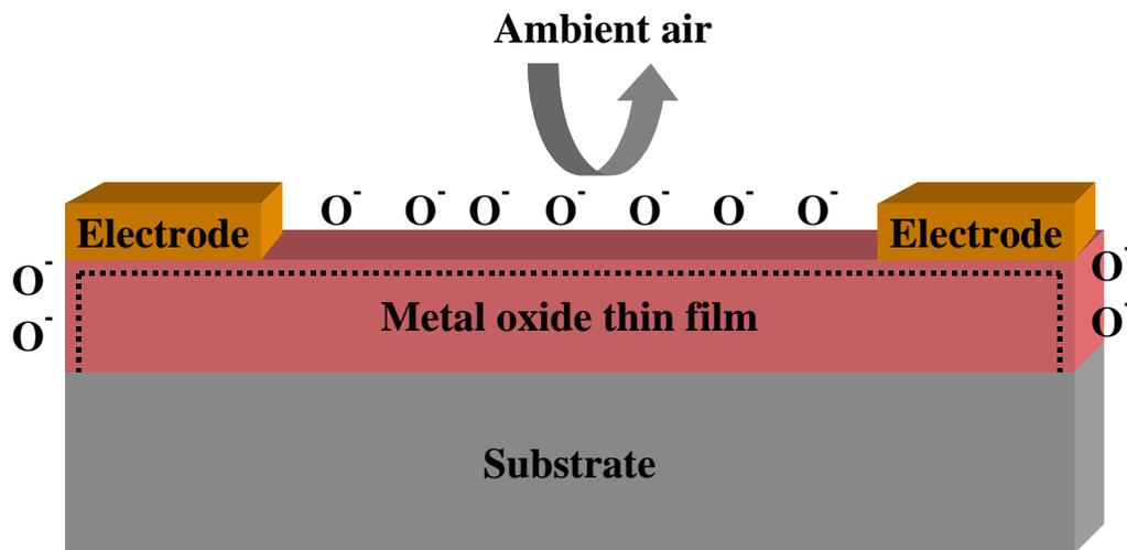
**Figure 1.1** – Schematic view of the semiconducting metal oxide surface with pre-adsorbed oxygen ions upon exposure to ambient air. The dotted line represents the space-charge layer formed close to the surface where the semiconductor is depleted of electrons.
