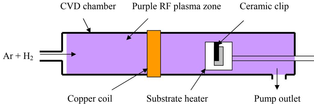
**Figure 3.2** – Schematic diagram of experimental setup
