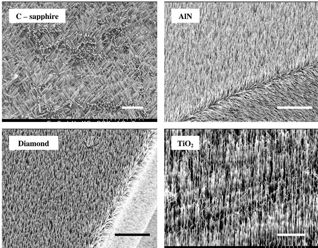
**Figure A4** – Epitaxial growth of ZnO nanowires on various substrates. Scale bars represent 5 μm.
