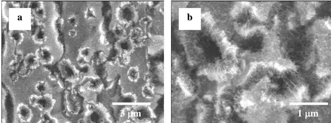
**Figure 2.12** – Vertically aligned CNT forests grown directly on a microhotplate. The nanotubes completely covered the sensor pads.
