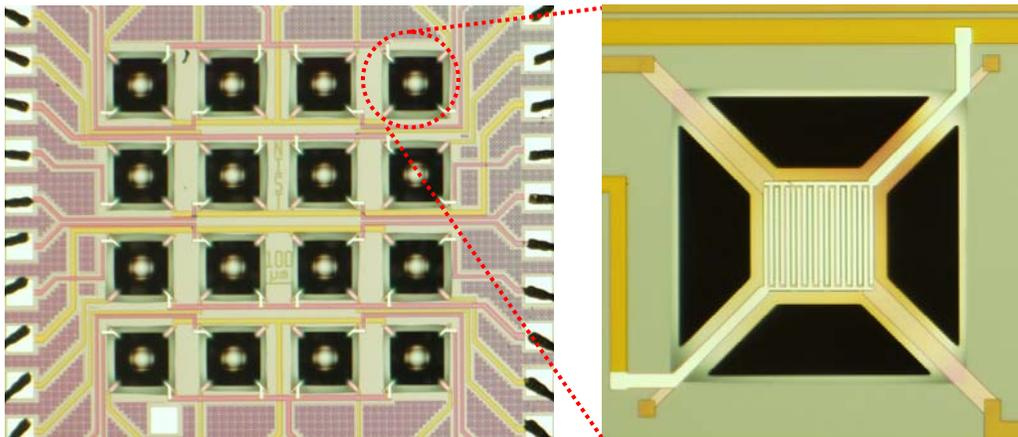
**Figure 2.11** – Optical images of a 16-element microhotplate array and a single microhotplate consisting of interdigitated comb-like contact pads (Distance between pads  $\approx 2 \mu\text{m}$ )
