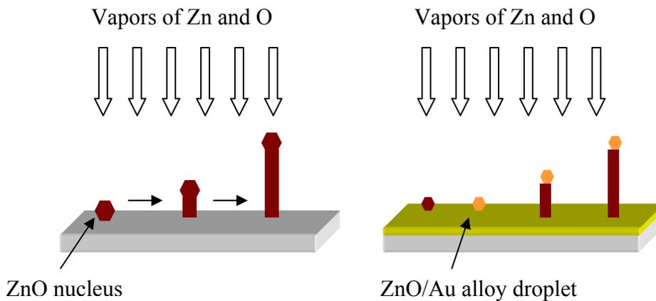
**Figure 4.7** – Non-catalytic V-S and catalytic VLS growth mechanisms of ZnO nanowires grown by chemical vapor transport.
