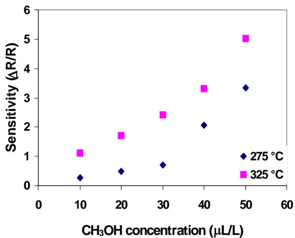
**Figure 4.17** – Sensitivity of the nanowire array to methanol, evaluated at 275 and 325 °C.
