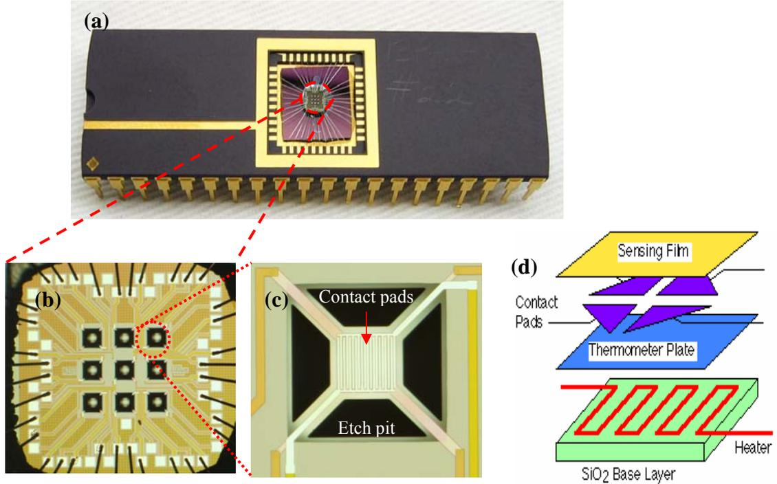
**Figure 2.3** – (a) Digital photograph of a package containing a 9-element array of microhotplates; (b), (c) Optical micrographs of microhotplates; (d) Multi-layered structure of an individual microhotplate device
