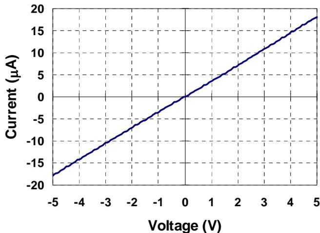
**Figure 4.14** – I-V characteristic of the device following repeated heat treatments at temperatures up to 350 °C.
