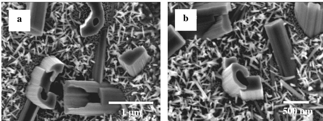
**Figure 3.13** – Irregular hollow nanostructures and solid nanorods observed to grow on a tungsten surface heated to 550 °C in RF Ar/CO plasma.
