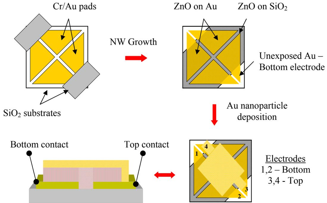
**Figure 4.10** – Schematic diagram of gas sensing device fabrication steps. The bottom images represent side and top views of the device.
