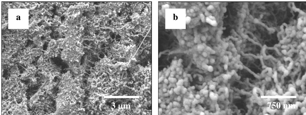
**Figure 2.13** – SnO<sub>2</sub> nanotube surface following SnO<sub>2</sub> CVD and removal of CNT templates
