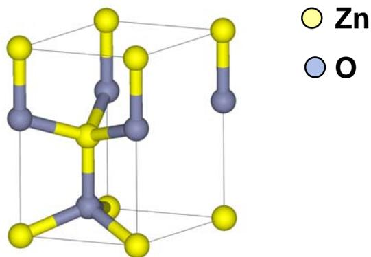
**Figure 4.1** – Wurtzite crystal structure of ZnO
