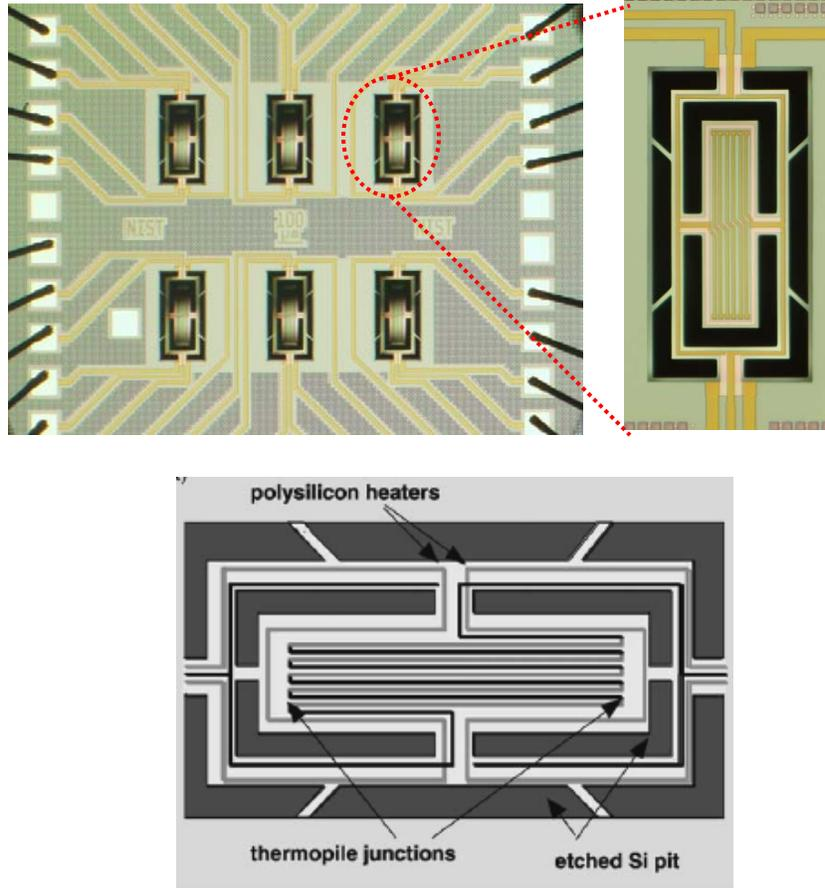
**Figure A1** – Optical images of a 6-element array of micro-calorimeters integrated on a chip and a closer look at an individual micro-calorimeter are shown on top. A schematic diagram of the device configuration is shown below.
