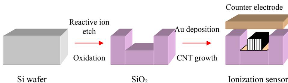
**Figure A3** – Schematic of steps involved in fabrication of CNT-array based gas-ionization sensor. Both trench depth and CNT lengths can be controlled to precisely adjust inter-electrode gap through this approach.
