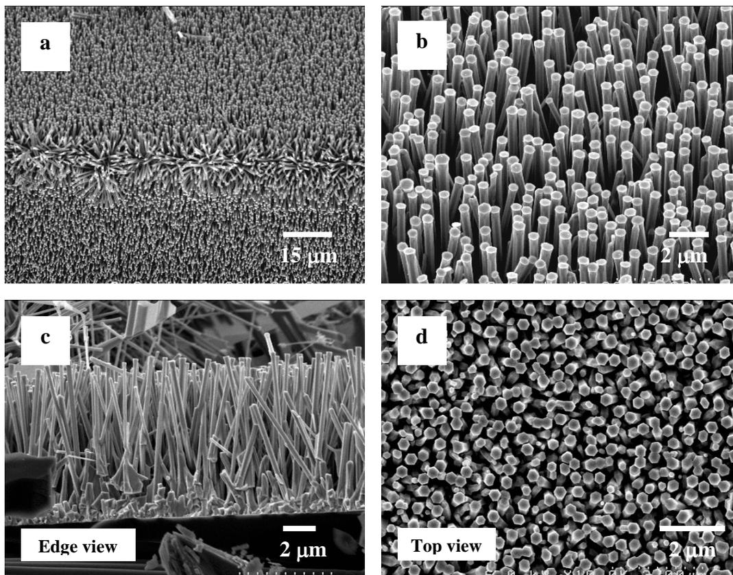
**Figure 4.2** – Aligned ZnO nanowire arrays grown directly on a Si wafer at 550 °C. (a) and (b) represent images of nanowires from a 45° perspective.
