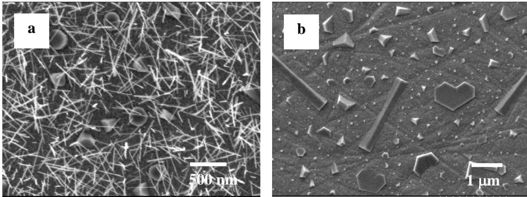
**Figure 3.5** – (a) Nanowires and crystallite structures grown by heat treatment of tungsten film at 600 °C in RF Ar/H<sub>2</sub> plasma. (b) Solid nanorods and other crystallite structures grown at 650 °C in RF Ar/H<sub>2</sub> plasma.
