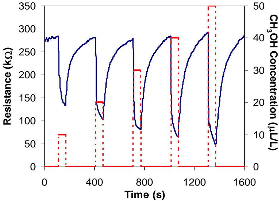
**Figure 4.15** – Sensor responses from the nanowire arrays at 325 °C to varying concentration of methanol (10 – 50 ppm).
