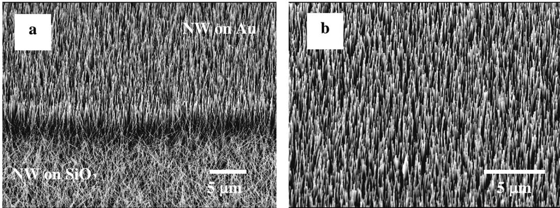
**Figure 4.11** – SEM images of gas sensing device sample surface. Vertically aligned nanowire grew on Au catalyst pads while randomly oriented nanowires grew on SiO<sub>2</sub>
