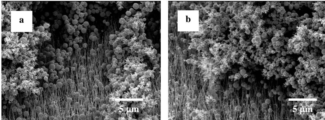
**Figure 4.9** – SEM images of Ag nanoparticles resting above the ZnO nanowire array imaged from a 45° perspective.
