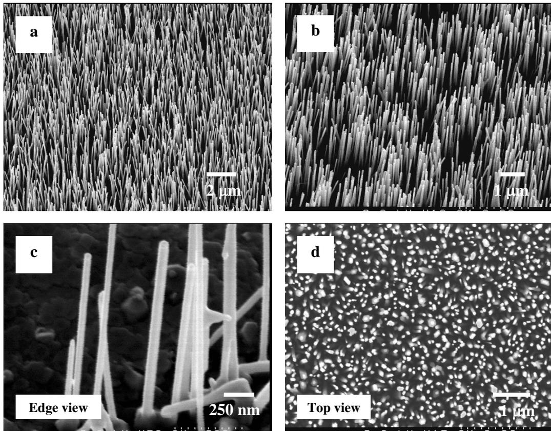
**Figure 4.3** – Aligned ZnO nanowire arrays grown on Au coated Si wafers at 550 °C. (a) and (b) were imaged from a 45° perspective.
