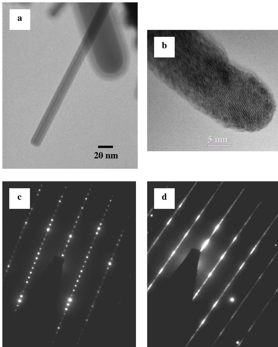
**Figure 3.9** – (a,b) Low and high resolution TEM images of W nanowires. (c,d) Electron diffraction patterns arising from 2 different nanowires.
