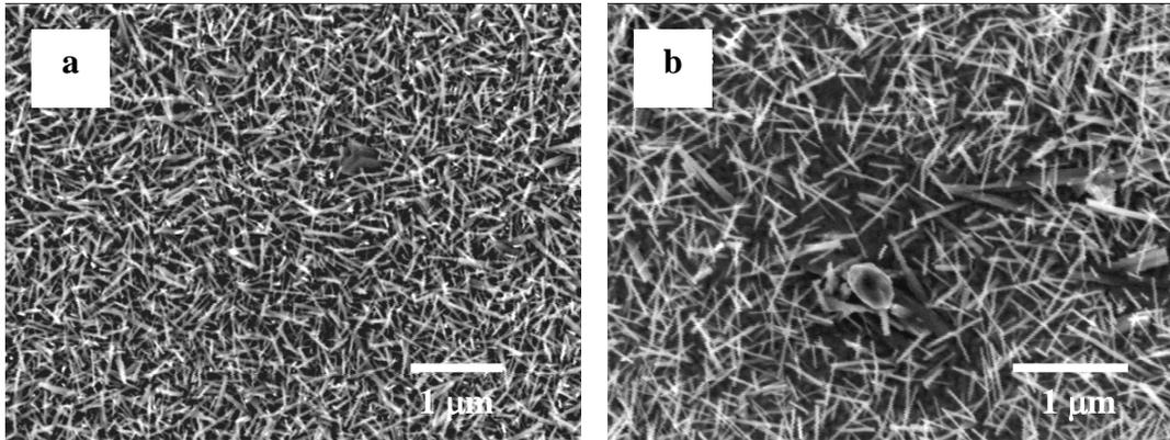
**Figure 3.12** – Uniform network of nanowires grown by heating a tungsten film to 550 °C in RF Ar/CO plasma.
