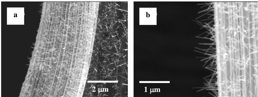
**Figure 3.8** – Nanowires grown on the surface of tungsten TEM grids heated at 550 °C in RF Ar/H<sub>2</sub> plasma.
