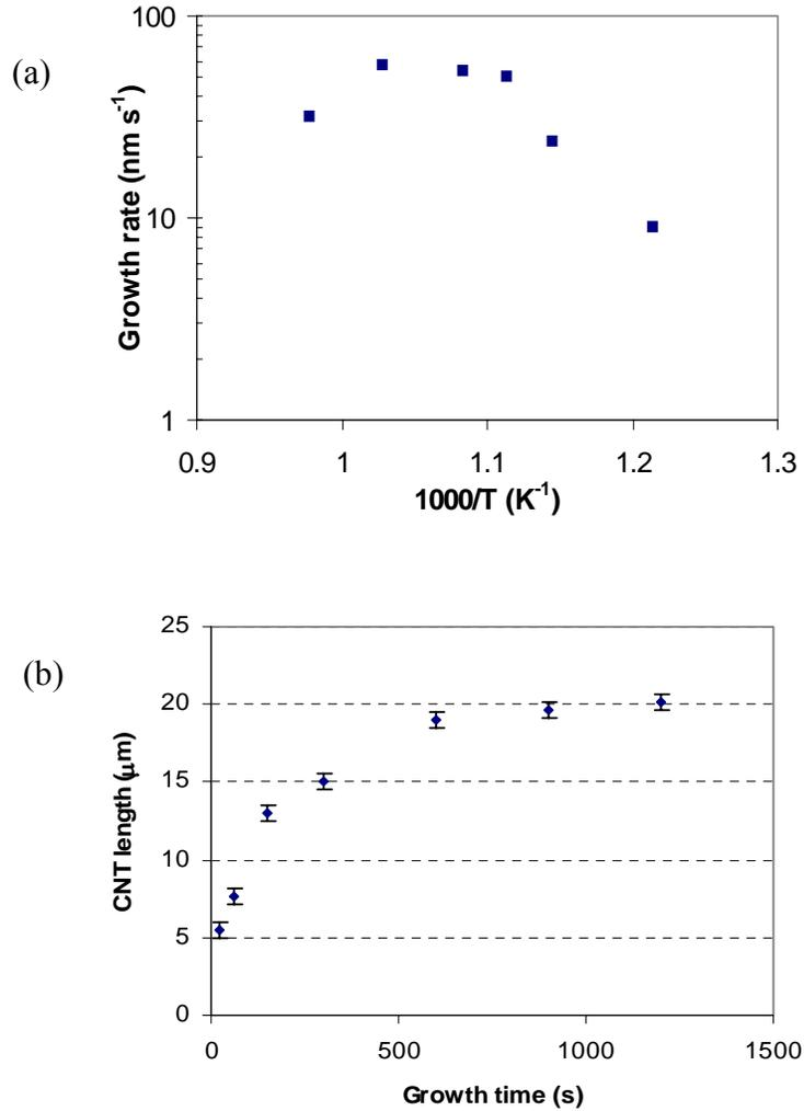
**Figure 2.10** – Influence of growth temperature (a) and growth time (b) on CNT array lengths. Temperature for growth time study = 620 °C.
