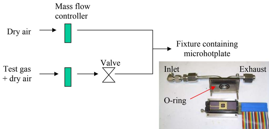
**Figure 2.14** – Schematic representation of gas-sensing measurement setup
