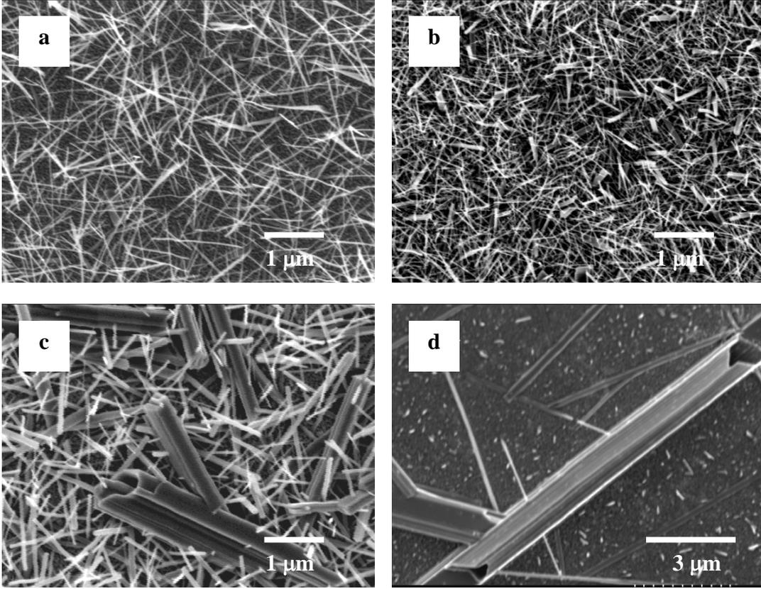
**Figure 3.11** – Schematic illustration of clip-substrate assembly used for mass-transfer dependence study. SEM images depict nanostructures grown in the regions indicated along the length of the substrate. (From left edge, a = 2 mm, b = 6 mm, c = 8.5 mm, d = 9.5 mm)
