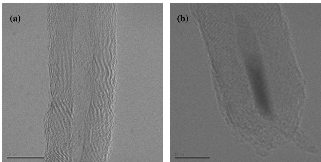
**Figure 2.9** – High-resolution TEM images of a single multi-walled CNT (grown on Au) clearly represent highly crystalline graphene sheets overlapping a hollow core. An oblong catalyst particle could be found on the tips of a few CNTs. The scale bars represent 10 nm.
