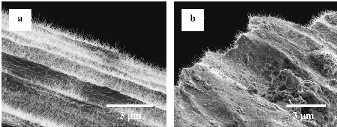
**Figure 3.7** – Nanowires grown on the surface of a commercial tungsten wire heated at 550 °C in RF Ar/H<sub>2</sub> plasma. Some nanowires extend out from the edge of the wire.
