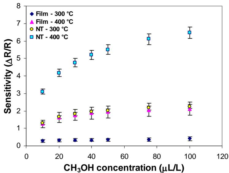
**Figure 2.16** – Sensitivity plots of microhotplate surfaces covered with SnO<sub>2</sub> nanotubes (NT) and bare SnO<sub>2</sub> thin films at 300 and 400 °C to varying concentrations of methanol.
