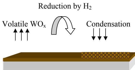
**Figure 3.10** – Vapor-solid growth mechanism of  $\text{WO}_x$  nanowires
