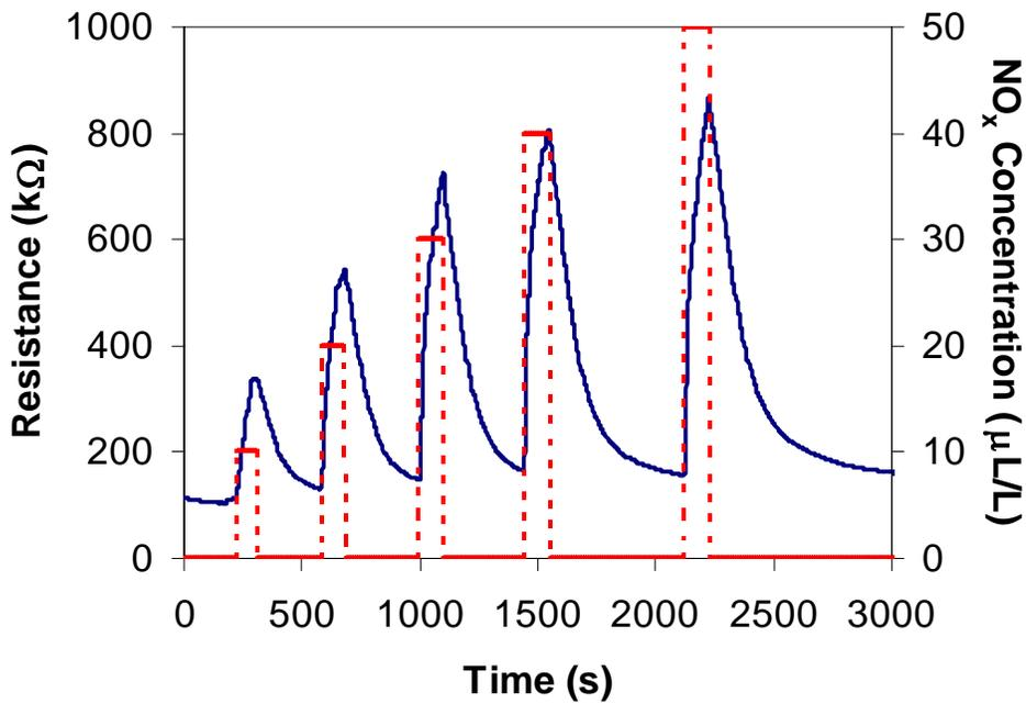
**Figure 4.16** – Sensor responses from the nanowire arrays at 325 °C to varying concentration of nitrous oxide (10 – 50 ppm).
