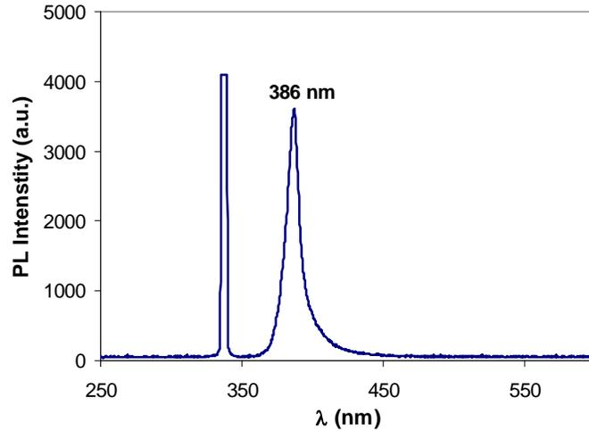
**Figure 4.6** – Room-temperature PL spectrum collected from Au catalyzed ZnO nanowire arrays on Si. The 338 nm peak corresponds to the exciting N<sub>2</sub> ion laser while the 386 nm peak is recorded from the ZnO nanowires.
