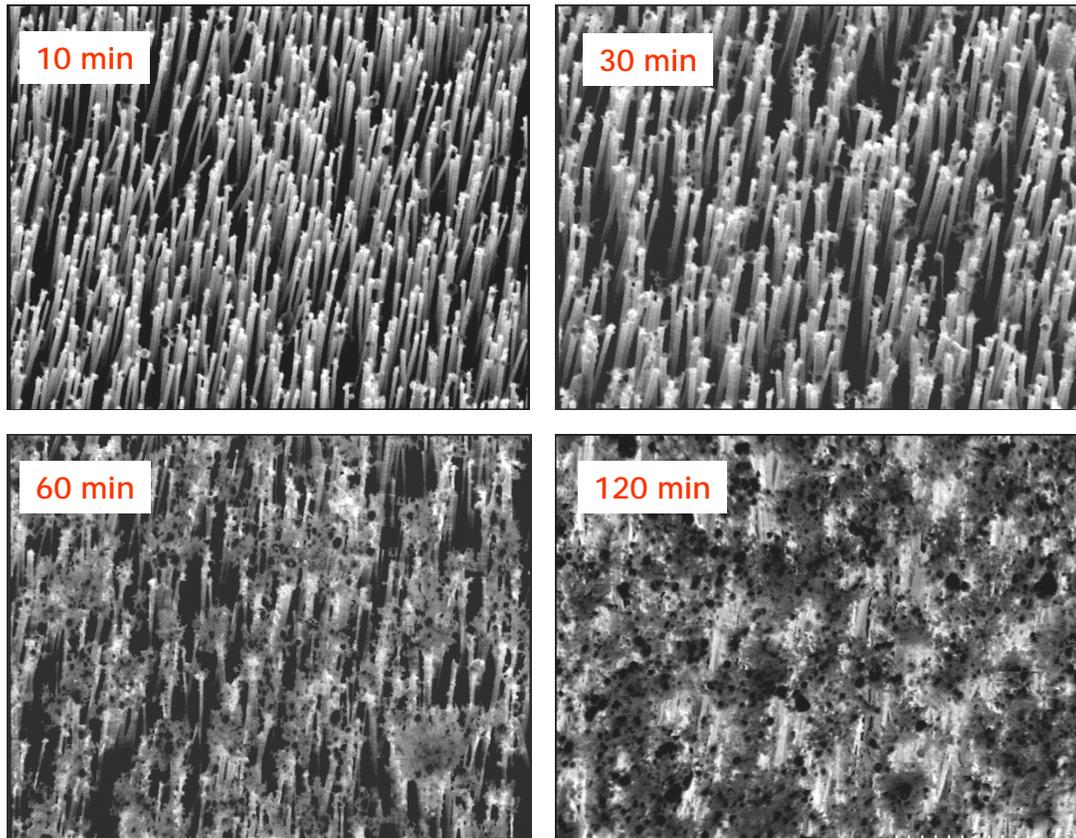
**Figure 4.12** – Evolution of Au nanoparticle film top contact at various stages of deposition.
