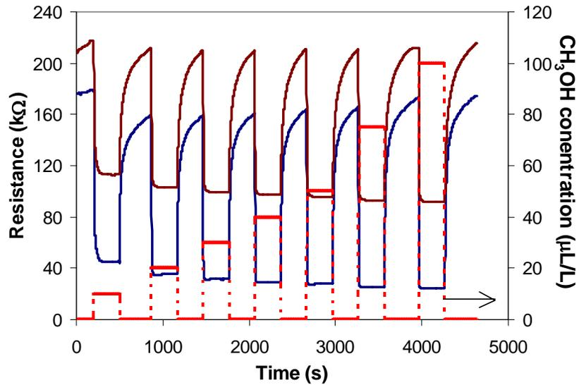
**Figure 2.15** – Typical gas sensing responses measured from a SnO<sub>2</sub> nanotube covered microhotplate sample to varying concentrations of methanol (red, axis on the right) at 300 °C (brown, top) and 400 °C (blue, bottom).
