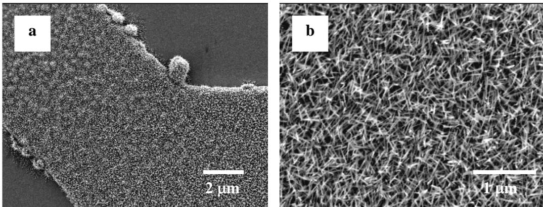
**Figure 3.15** – SEM images of tungsten oxide nanowires grown on a microhotplate
