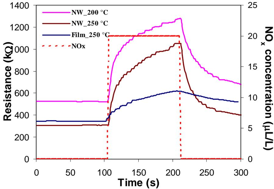
**Figure 3.16** – Gas sensing responses to 20 ppm  $\text{NO}_x$  recorded from  $\text{WO}_3$  nanowires and a  $\text{WO}_3$  thin film
