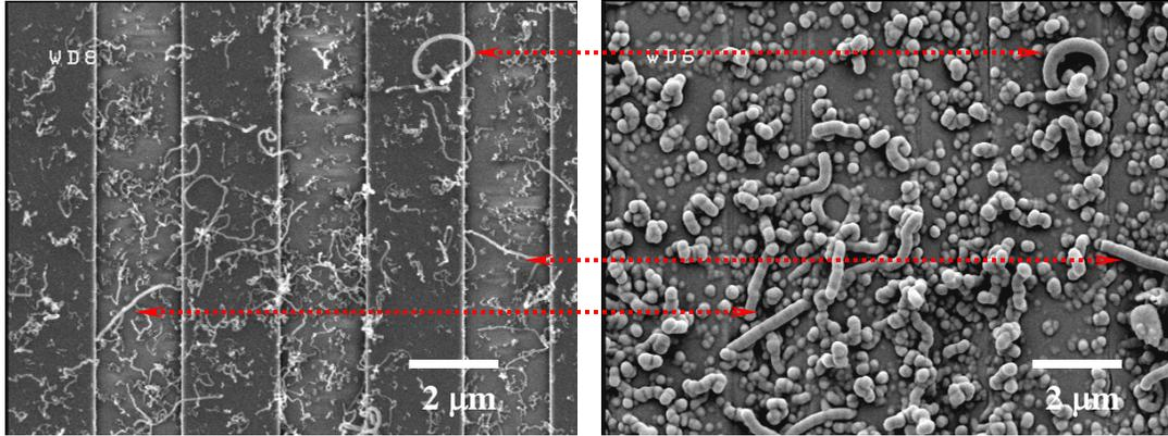
**Figure 2.6** – SEM images of microhotplate surface before and after SnO<sub>2</sub> deposition. The arrows indicate specific shapes on the surface that were imaged to verify conformal coating.
