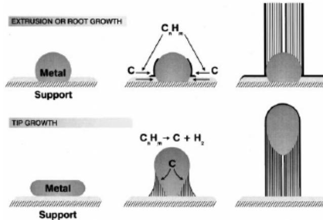
**Figure 2.2** – Root and tip growth modes for carbon nanotubes. Reproduced from Ref. [50].
