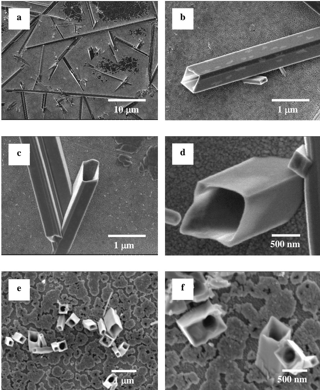
**Figure 3.6** – Hollow, square microducts observed to grow in the certain specific regions of the substrate. (a-d) and (e-f) represent ducts grown on 2 different samples. Some of the ducts were several hundred microns long.
