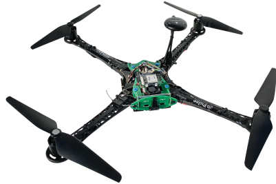
ModalAI VOXL 2 m500 quadcopter platform [Credit: ModalAI]
