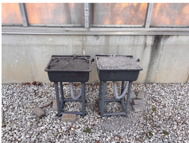
Figure 5.2.1 Field lysimeters containing Caster slag (left) and EAF slag (right), installed outdoors at the University of Maryland for the field exposure experiment, December 2025 - May 2026. Leachate was collected through the drainage outlet at five sampling intervals over the monitoring period.
