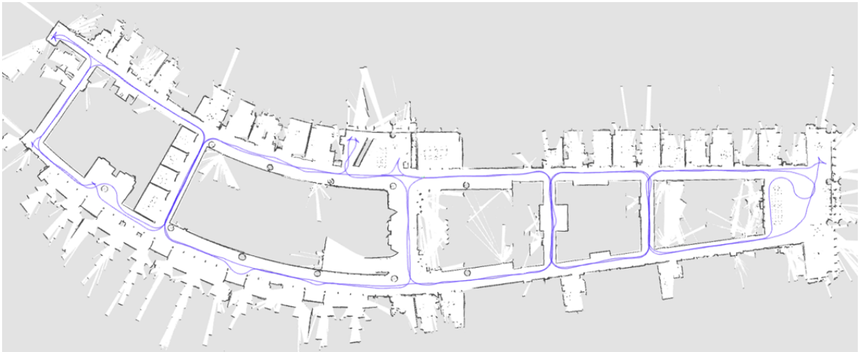
Figure 4.5: Default Cartographer map from Building 1 with the robot path visualized in blue
