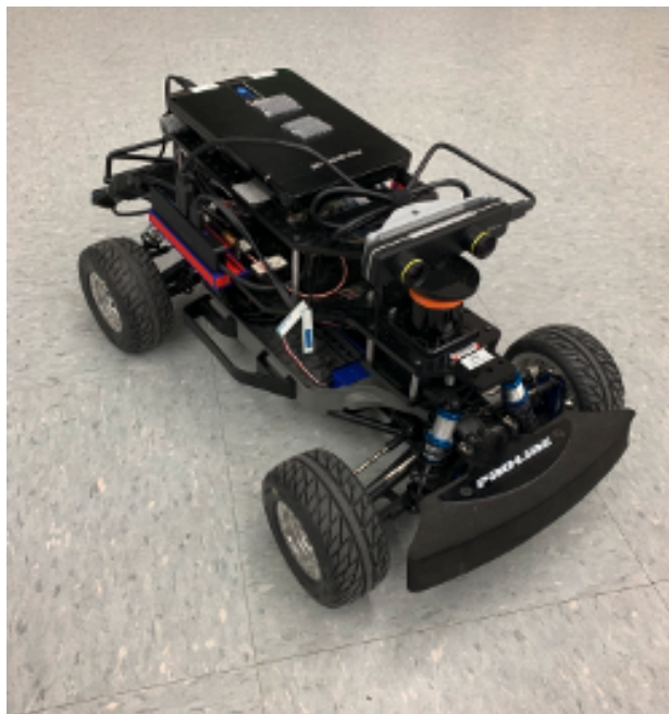
Figure 2.6: The RACECAR UGV
