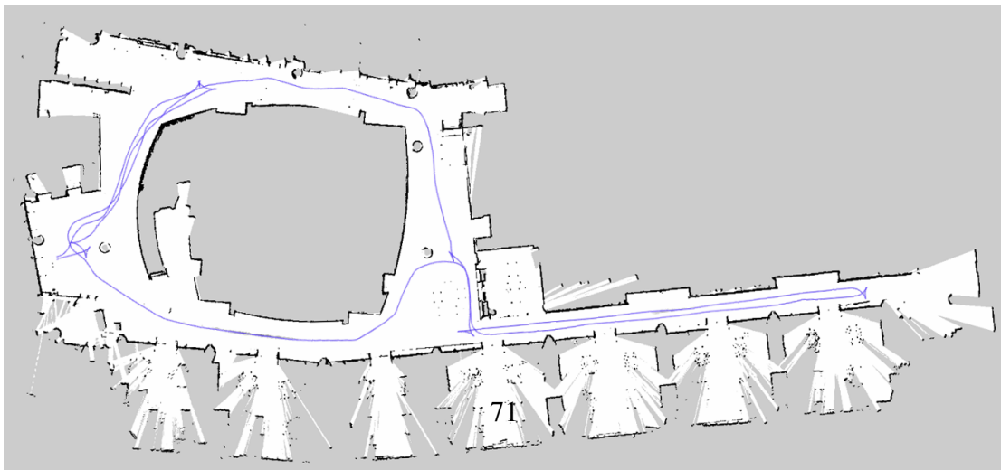
Figure 4.8: Cartographer map with standard setting for Building 2 with the robot path visualized
