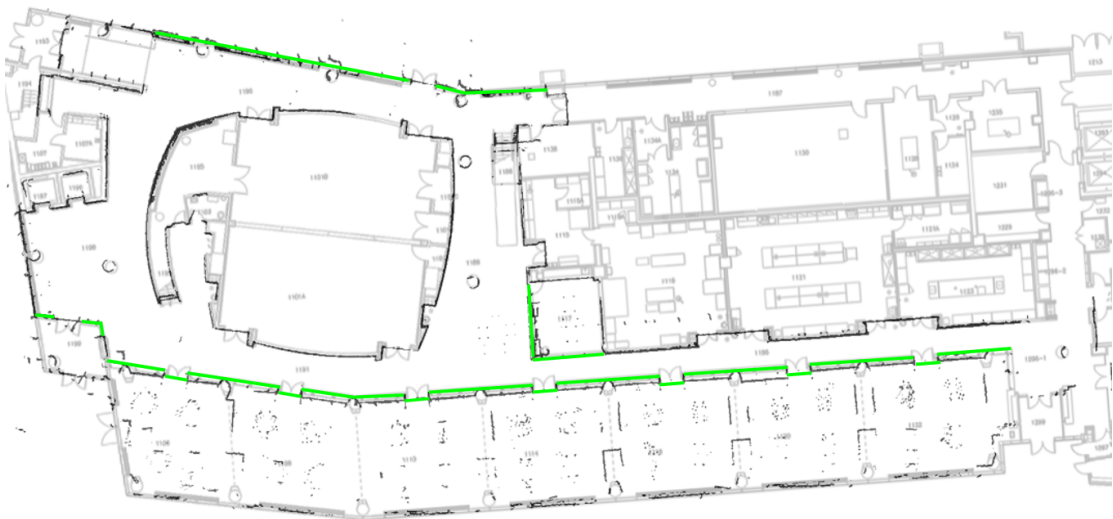
Figure 4.7: Cartographer map with standard setting from Building 2 overlaid with the floor plan with glass walls marked manually in green
