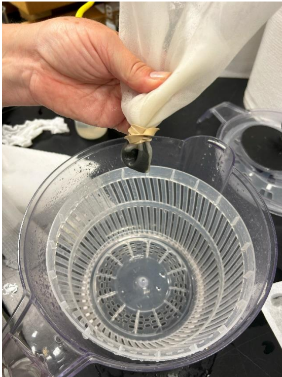
Image 3.1 Removal of excess water from M. wollei samples with use of salad spinner, to provide more consistent measurement of biomass wet weights among all samples.
