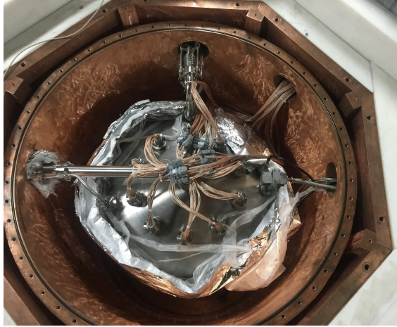
Figure 3.9: A top-view photo of feedthroughs passing through 4 ports on the Cu outer vessels.
