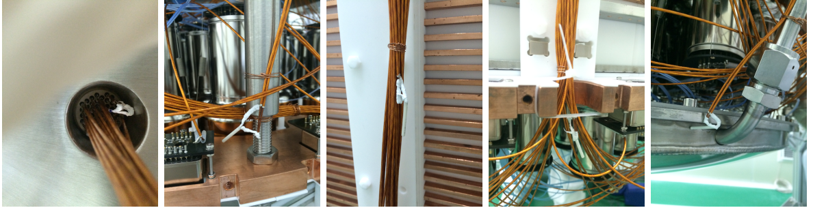
Figure 3.15: Five temperature sensors in PandaX-II detector top down.
