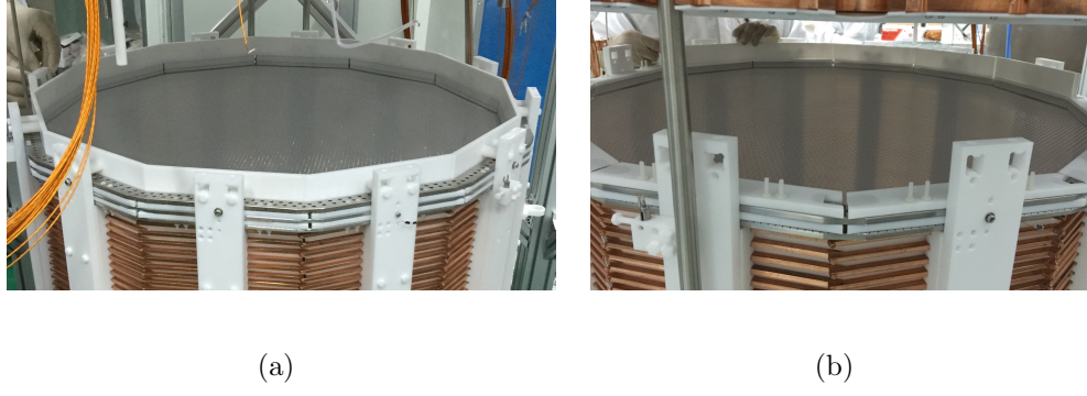
Figure 3.7: The original 3 electrodes (a) and the final 2 electrodes (b) on the top of PandaX-II TPC.
