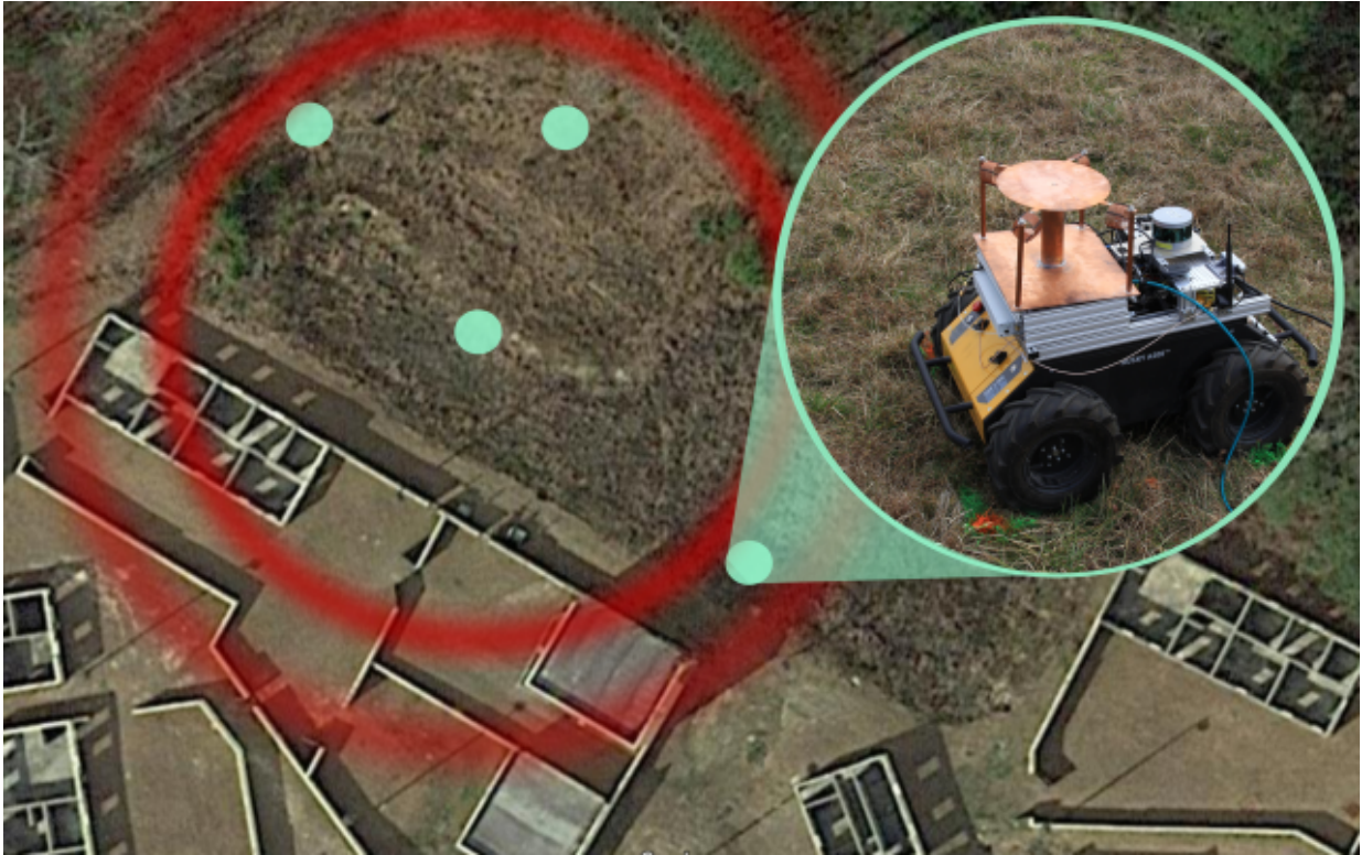
Figure 1.1: Several ground robots occupy a complex environment. The image zooms in on one of them to show its low-VHF antenna. The concentric circles around one of the robots show that it is radiating equally in all directions using this low-VHF antenna.
