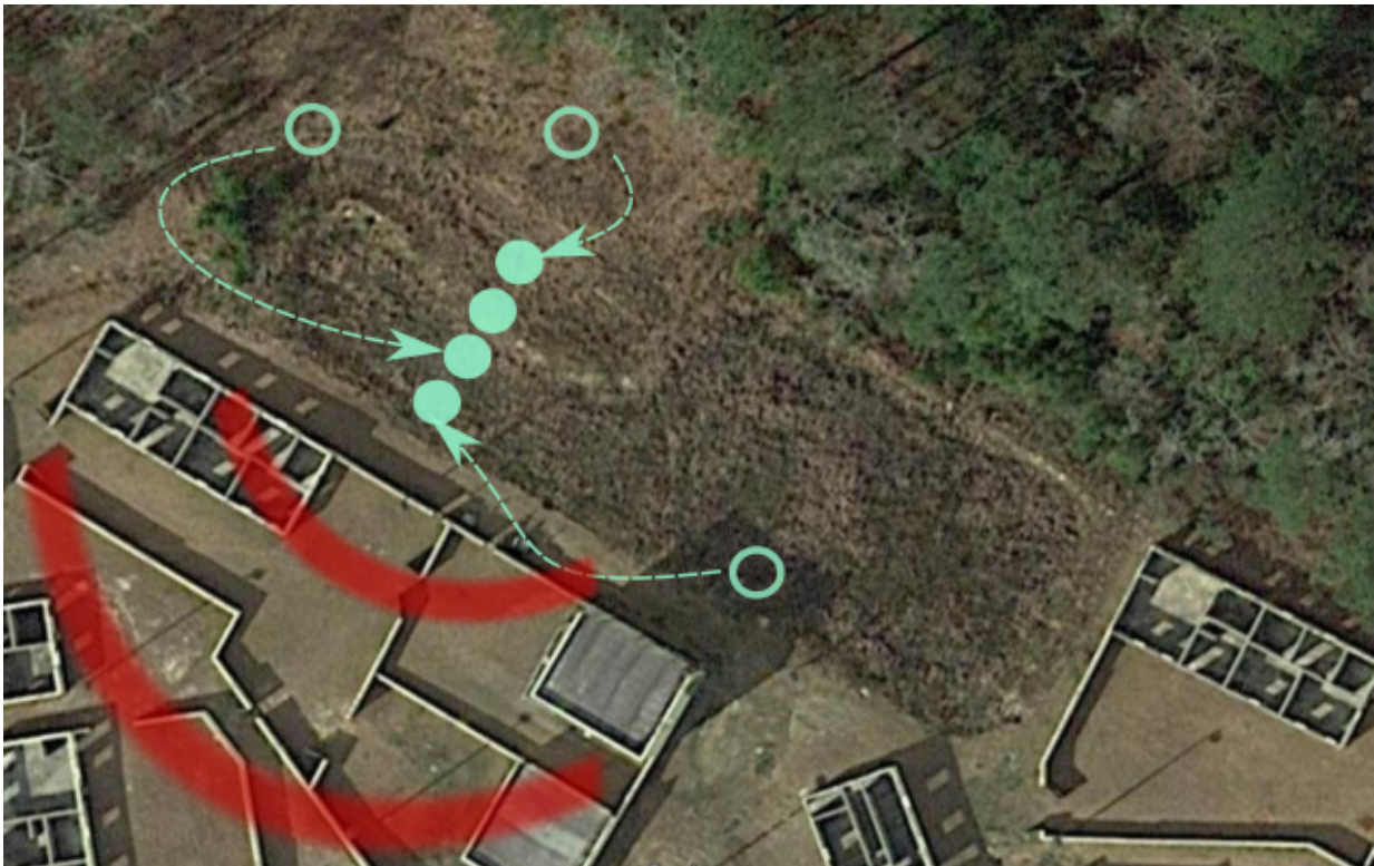
Figure 1.2: Several ground robots maneuver to form a robotic parasitic array to create a higher gain and more directional signal.
