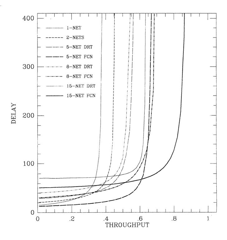
Figure 6: Throughput - Delay Caracteristics for 15-user slotted ALOHA system.
