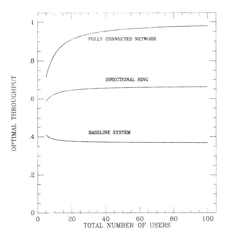
Figure 4: Optimal Throughput vs. total number of Users for slotted ALOHA
