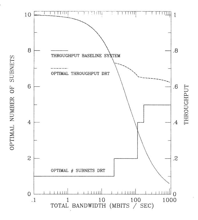
Figure 9: Optimal Number of Subnets and Optimal Throughput vs.
