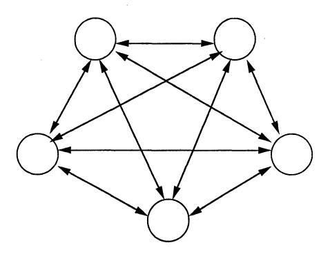
Figure 3(a): The Fully Connected Network
