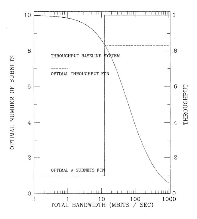
Figure 10: Optimal Number of Subnets and Optimal Throughput vs.
