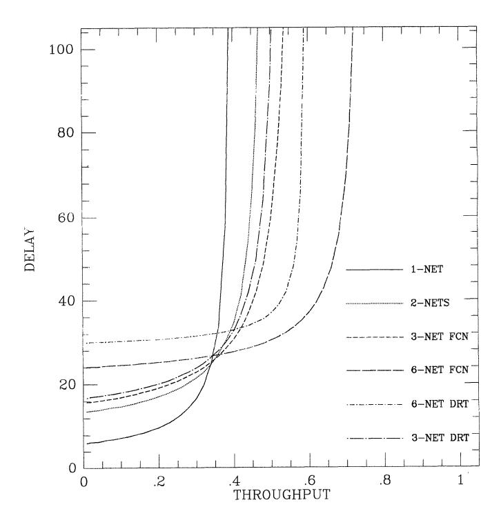
Figure 5: Throughput - Delay Caracteristics for 6-user slotted ALOHA system.
