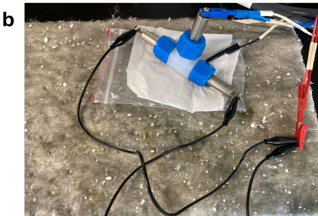
Fig. 4.3. (a) Schematic diagram of the circuit connection for presodiation of both V_2O_5 electrodes. The two V_2O_5 electrodes of the T-cell are short and connected to the potentiostat to be sodiated to the same extent. (b) Picture of T-cell and the corresponding circuit for presodiation.
