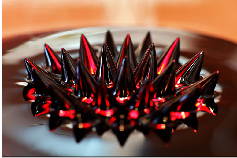
Figure 4.8: Real experiment of a ferrofluid subject to a non-uniform magnetic field. Courtesy (reproduced with permission, see Appendix) of [140].
